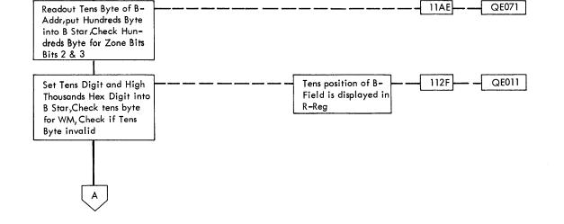
1400 Tape Operation-Tapes on MPX Channel or Selector Channel--I Cycles RS Chart 11 (Sheet 1)
