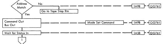
1400 Compatibility-Tapes on MPX Set Up--Tape Write Op 9 Track Drive RS Chart 15 (Sheet 1)
