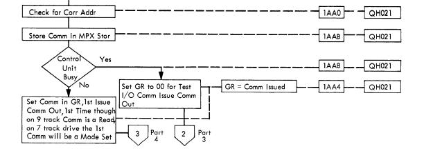
1400 Compatibility Tape Read Operation--Selector Channel RS Chart 12 (Sheet 1)
