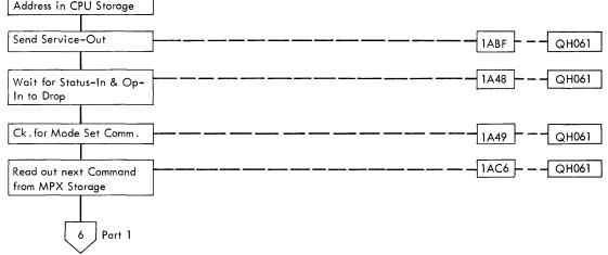
1400 Compatibility Tape Selector Setup-Tape Write Op 9 Track Drive RS Chart 13 (Sheet 2)
