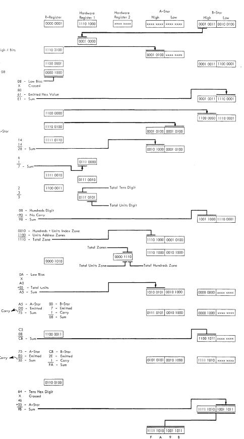
Test Total Hundreds Zone to Determine Correct Hex Digits to Add to High A-Star and High B-Star. For this Example Bits are 10 (Hex Digits are 7D0). Add D0 to High A-Star, Any Carry from A-Star is Added to High B-Star. Add the 7 to High B-Star.
