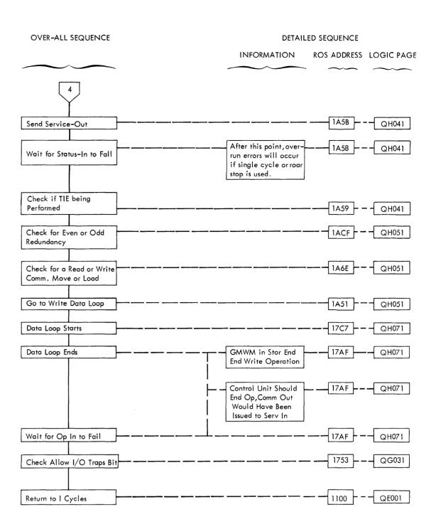
1400 Compatibility Tape Selector Setup-Tape Write Op 9 Track Drive RS Chart 13 (Sheet 3)
