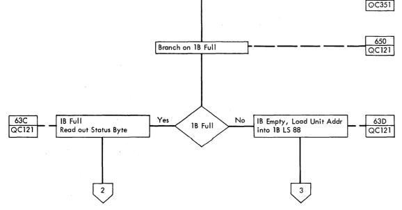
MPX--SIO Input/Output Burst or Byte Mode RS Chart 4 (Sheet 1)
