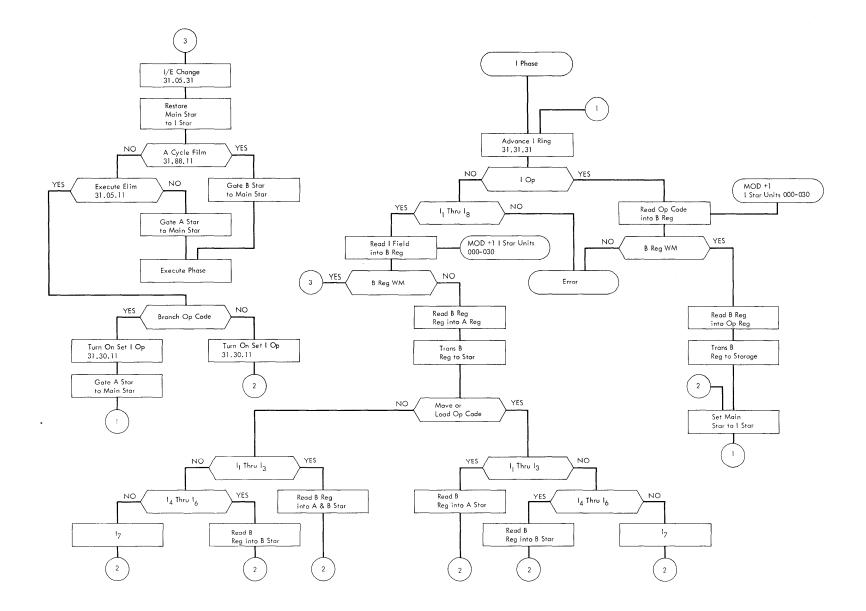
Example for A-Star or B-Star Address Development During I-Phase of 1401 Compatibility Feature on the 2030.
