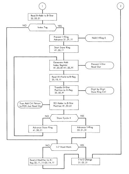
Example for A-Star or B-Star Development with Indexing During I-Phase of 1401 Compatibility Feature on the 2030. Program is for a 16,000 Positions of Storage 1401 and the 2030 Has 65,536 Positions of Storage .
