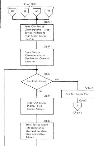
Load and Test; the Second Operand is Placed in the First Operand Location. Condition Codes are Set.
