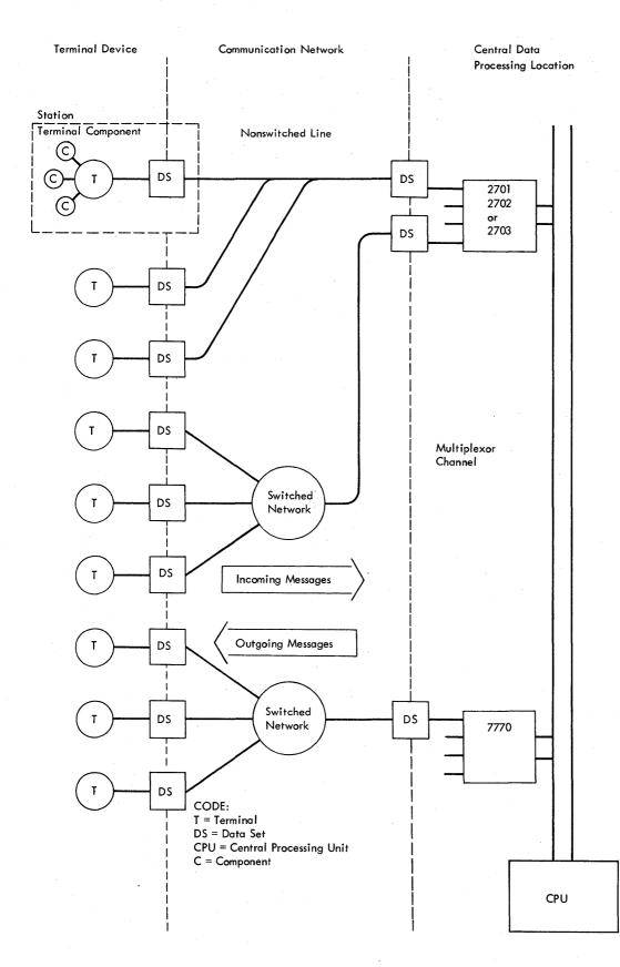
Figure 1. Configuration of a Communication System (Part 1 of 2) Start-Stop System
