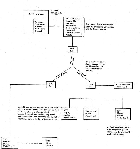
Figure 73. Remotely Attached 3270 Display System
