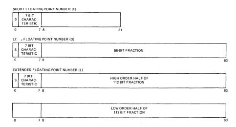
Figure 5-5. Floating-Point External Formats
