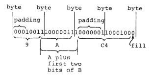
Figure 5-4. Bit-Length Specification (Multiple Operands)
