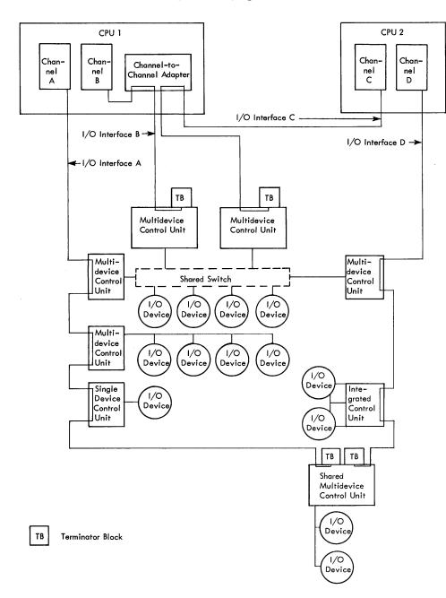
Figure 1. Input/Output Interface - Multiple Configurations
