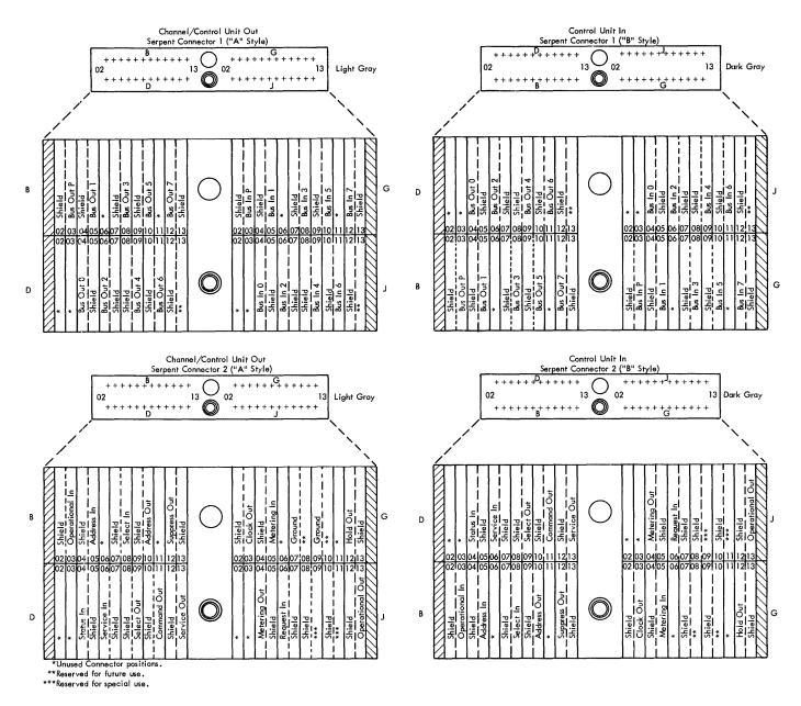
Figure 7. I/O Interface Connector Pin Assignments
