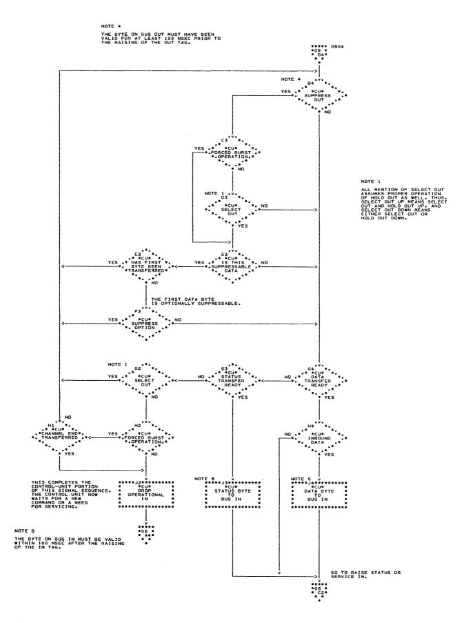
Flow Diagram 8. Burst Mode Waiting Loop
