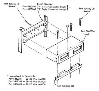
Figure 9. Panel Mount with Optional Strain Relief
