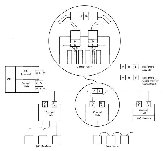
Figure 10. Off-Line Utilization
