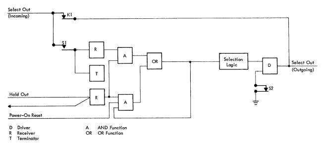
Figure 3. Representative Select-Out/Hold-Out Special Latch
