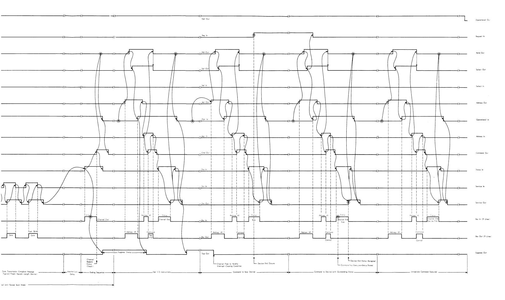
Sequence Chart 2. Control Unit Forced Burst Mode – Multiplexer Channel Appendix C. Supplementary Application Information C-13
