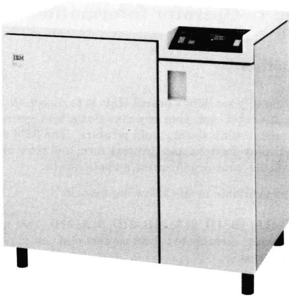
**Figure 1-1. IBM 3274 Control Unit Model 1A, 1B, 1D, 21A, 21B, 21D, 31A, 31D, 41A, or 41D**
