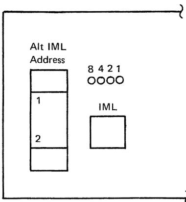
When the IML pushbutton is pressed, these lights are tested (they should all be on). When the IML pushbutton is released (or when the 3274 is initially powered on) the 3274 IML procedure is initiated.
