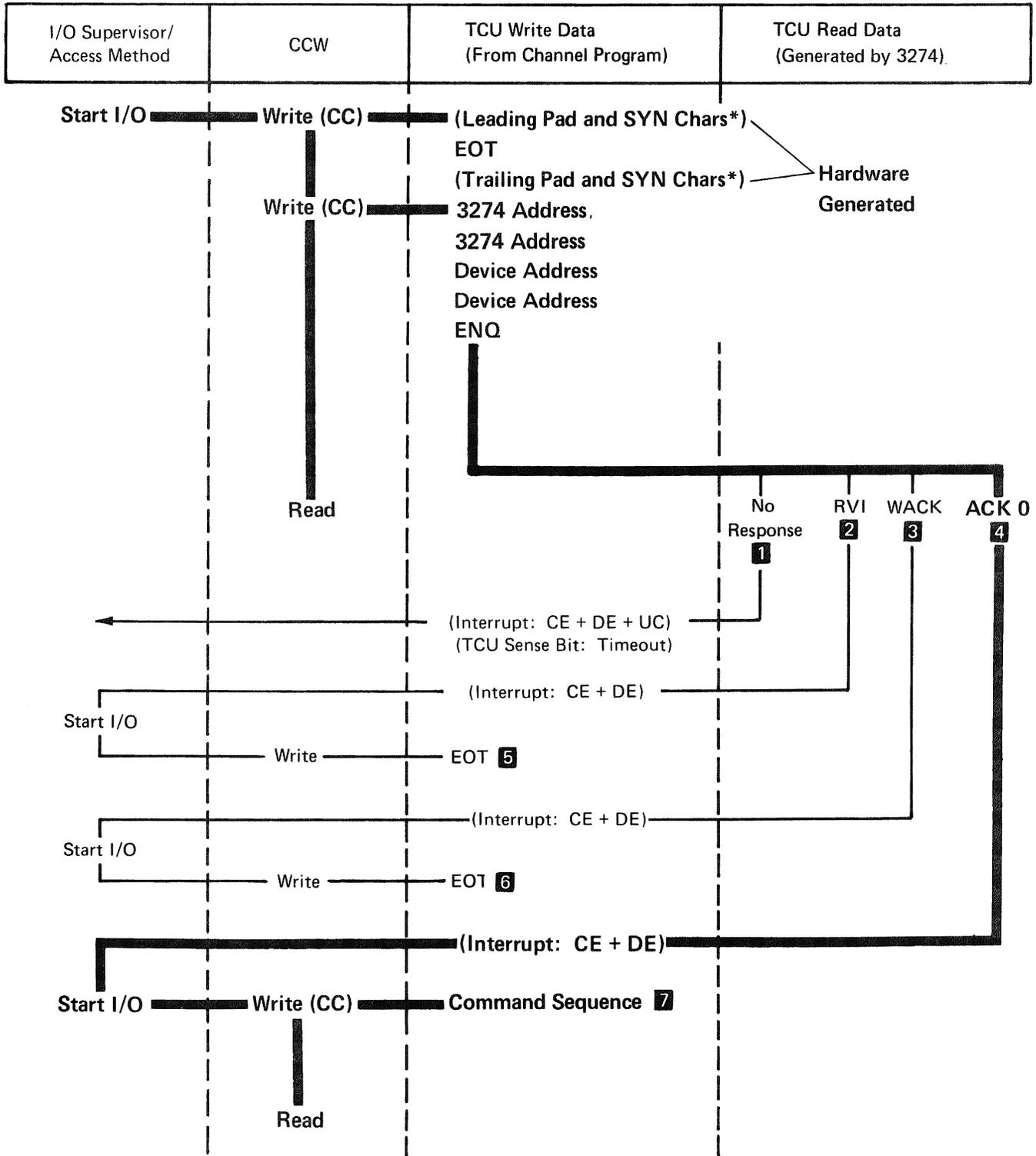
\*Only the critical framing characters (sync pattern and pad) are shown. All other framing characters are also hardware-generated as required. See SL *General Information – Binary Synchronous Communications*, GA27-3004, for a complete description.
