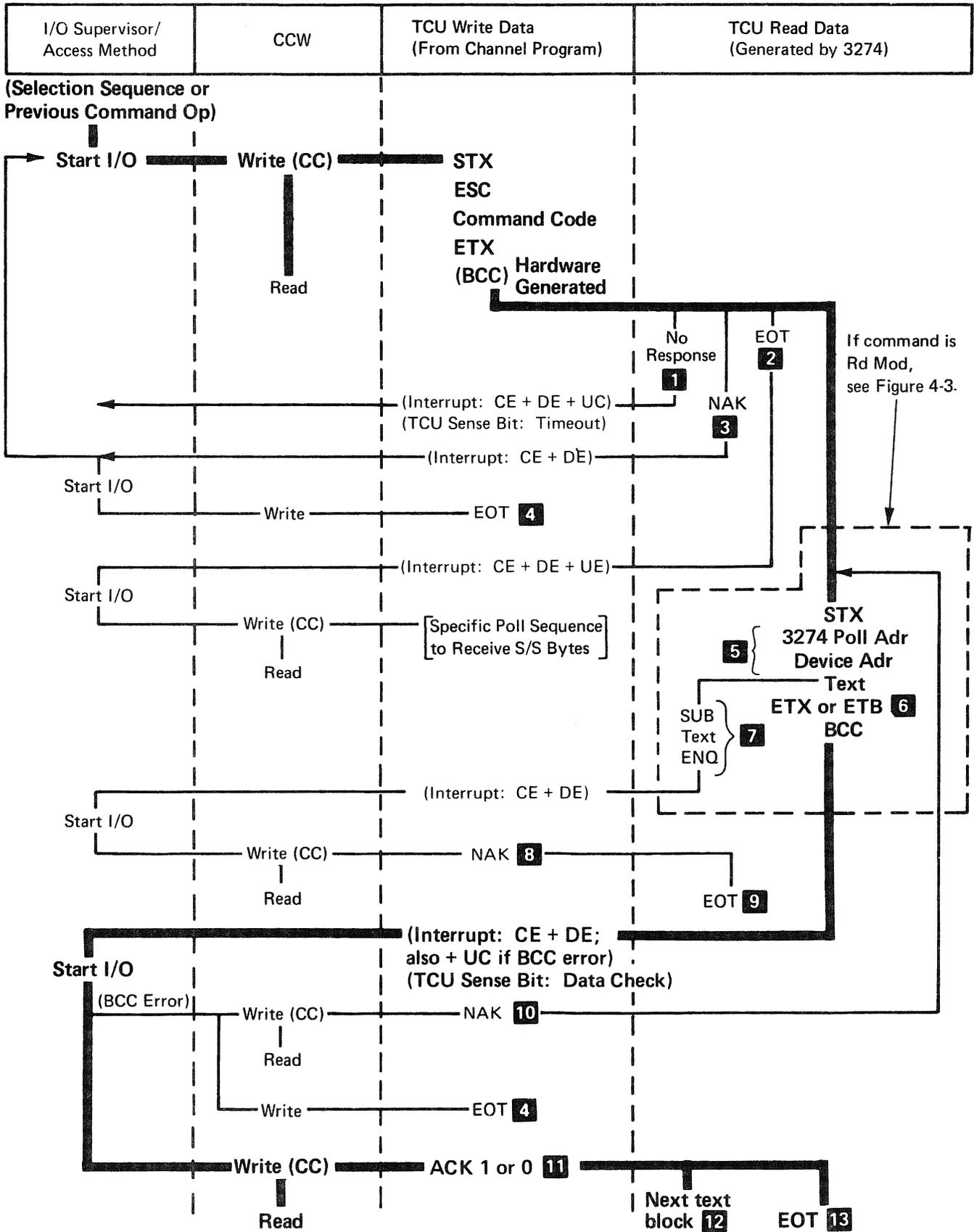
Figure 4-6 (Part 1 of 2). Read-Type Command, Sequence/Response Diagram
