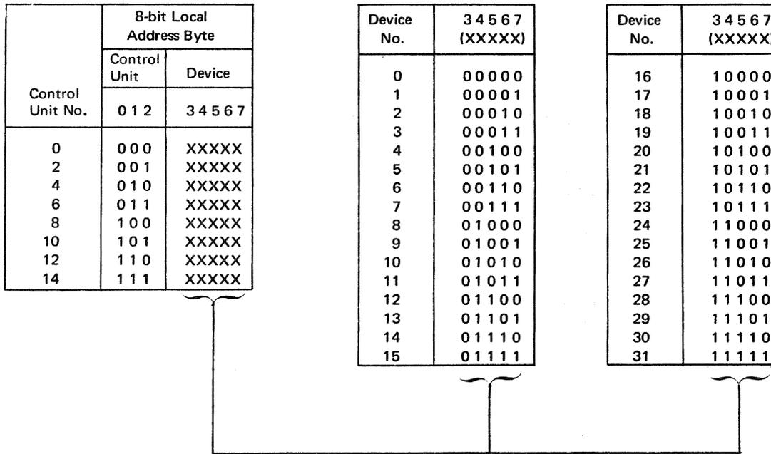
**Note:** Control Unit Nos. 1, 3, 5, 7, 9, 11, 13, and 15 cannot be assigned when attached devices are assigned Device No. 16 or greater.
