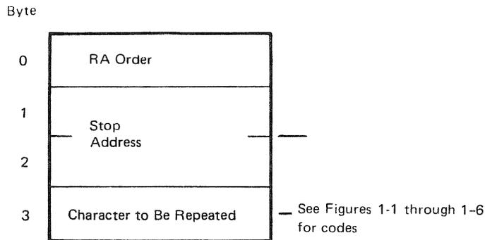
The third character following the RA order is always interpreted as the character that will be repeated. If an invalid stop address is specified, the write operation is terminated at this point without storing the character, and error status is generated. When Color, Extended Highlighting, or Programmed Symbols attributes are specified for the character, the attribute values are entered into the character attribute buffer as each repeated character is written in the data buffer.
