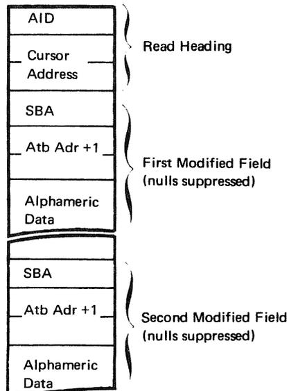
If a space or null selector-light-pen AID is generated, at a 3277 display, fields are not transferred to main storage during the read-modified operation. Instead, when a set MDT bit is found (indicating selector-light-pen and/or keyboard activity), only the Read Heading, the SBA order code, and the attribute address + 1 are transferred.
