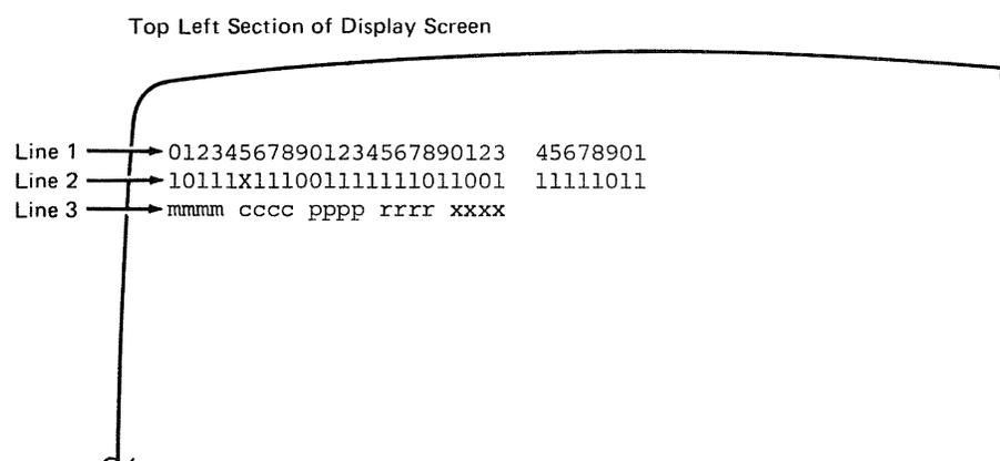
Line 1: Low-order digit of the port addresses configured on the 3274. When a Type B adapter is attached, the last (highest) Type A port and the first (lowest) Type B port are separated by two spaces on lines 1 and 2. The example shows 24 Type A terminals and eight Type B terminals.
