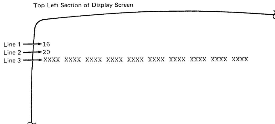
where xxxx xxxx . . . represents the 20 bytes of data (x = 1 byte). From left to right, the data is interpreted as follows:
