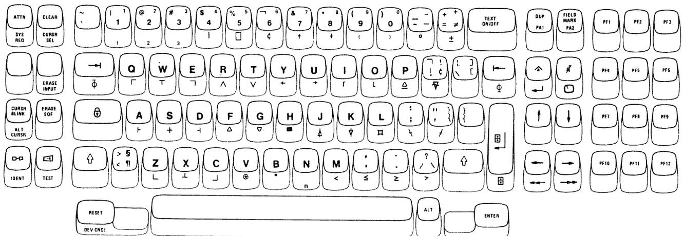
Figure D-10. 87-Key Typewriter/Text Keyboard
