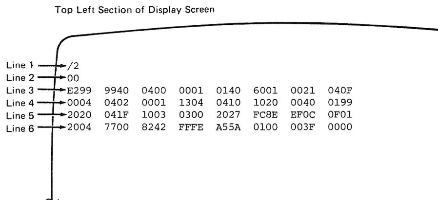
By pressing the ENTER key, the next 64 bytes of the configuration table will be displayed. Line 2 indicates the starting location of the first byte displayed. (The last (0) digit is dropped.)
