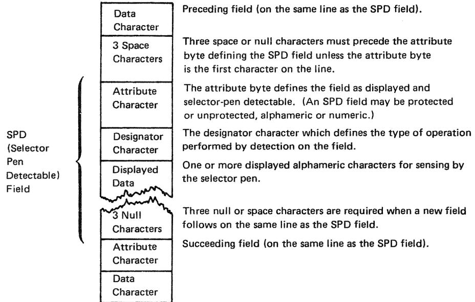
Figure 6-31. Definition of Field for Selector Pen Operation
