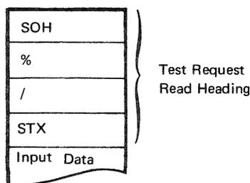
The Test Request Read heading is generated by the control unit. The remainder of the data stream is the same as described previously for read-modified operations, excluding the 3-byte read heading (AID and cursor address). If the
