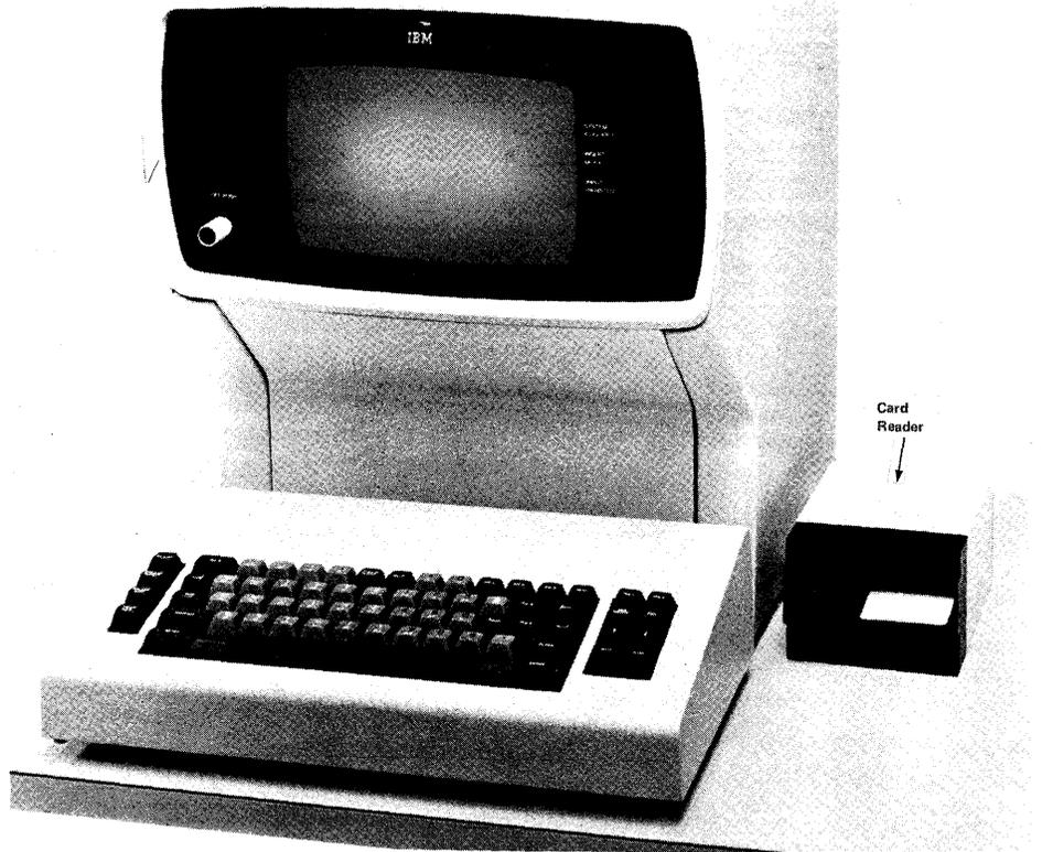
Figure H-6. Operator Identification Card Reader (3277 Attachment)
