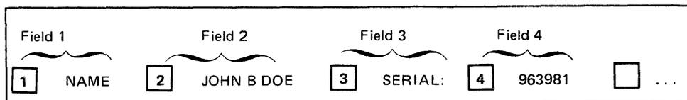
Figure 6-1. Example of Four Fields and Attribute Bytes
