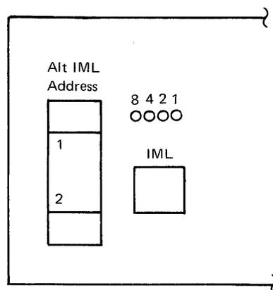
When the IML button is pressed, a test of these lights is performed (they should all be turned on). When the IML button is released (or when the 3274 is initially powered on) the 3274 IML procedure is initiated.
