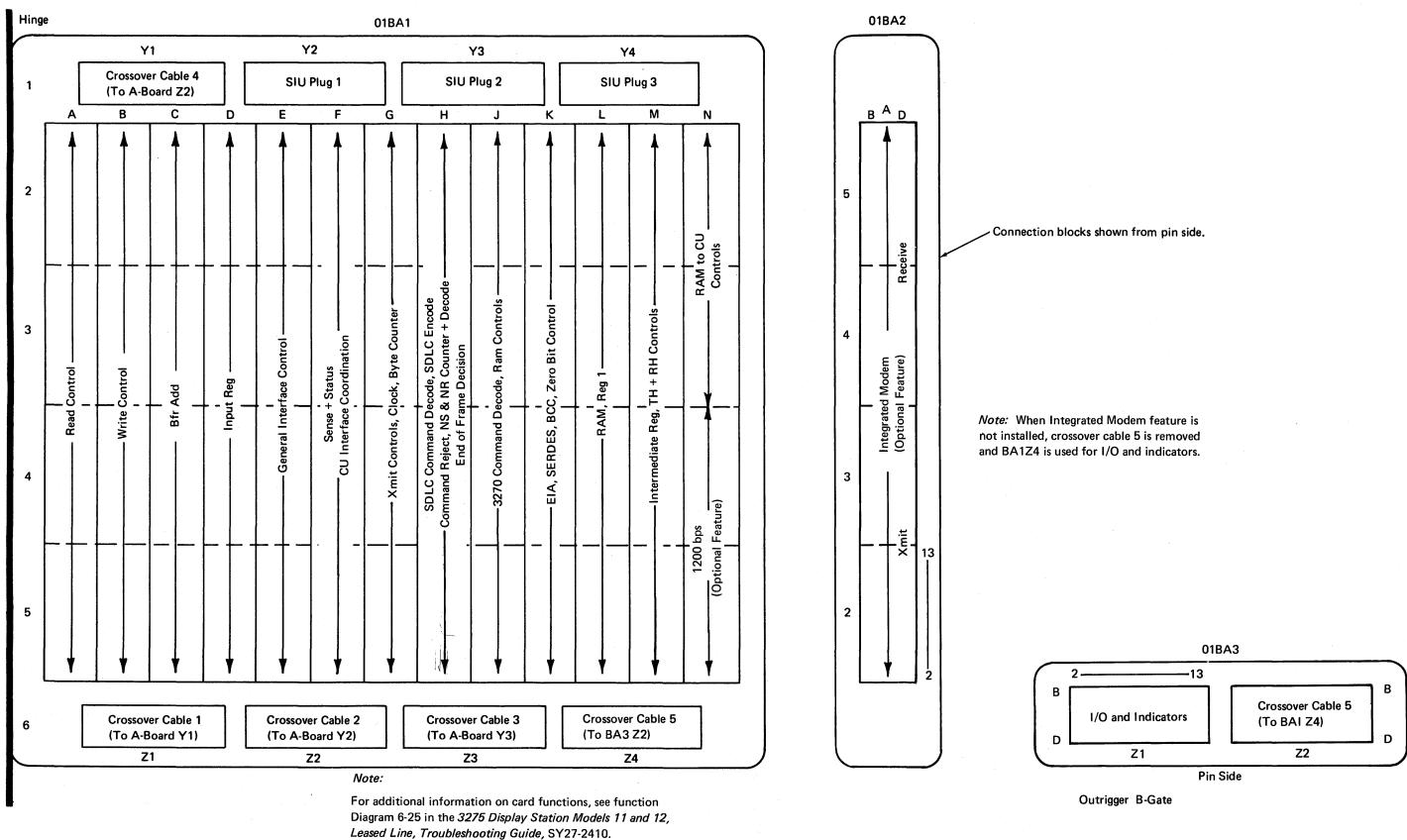
Diagram 4-17. B-Gate Card Layout by Function (Card Side)
