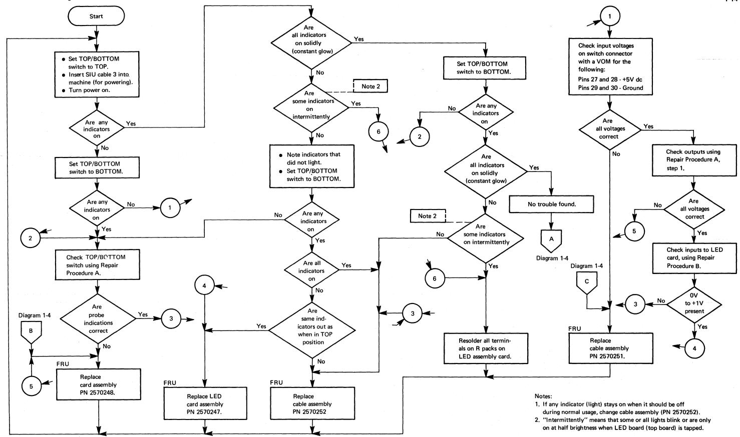
Diagram 1-3. SIU-LED Checkout Flowchart
