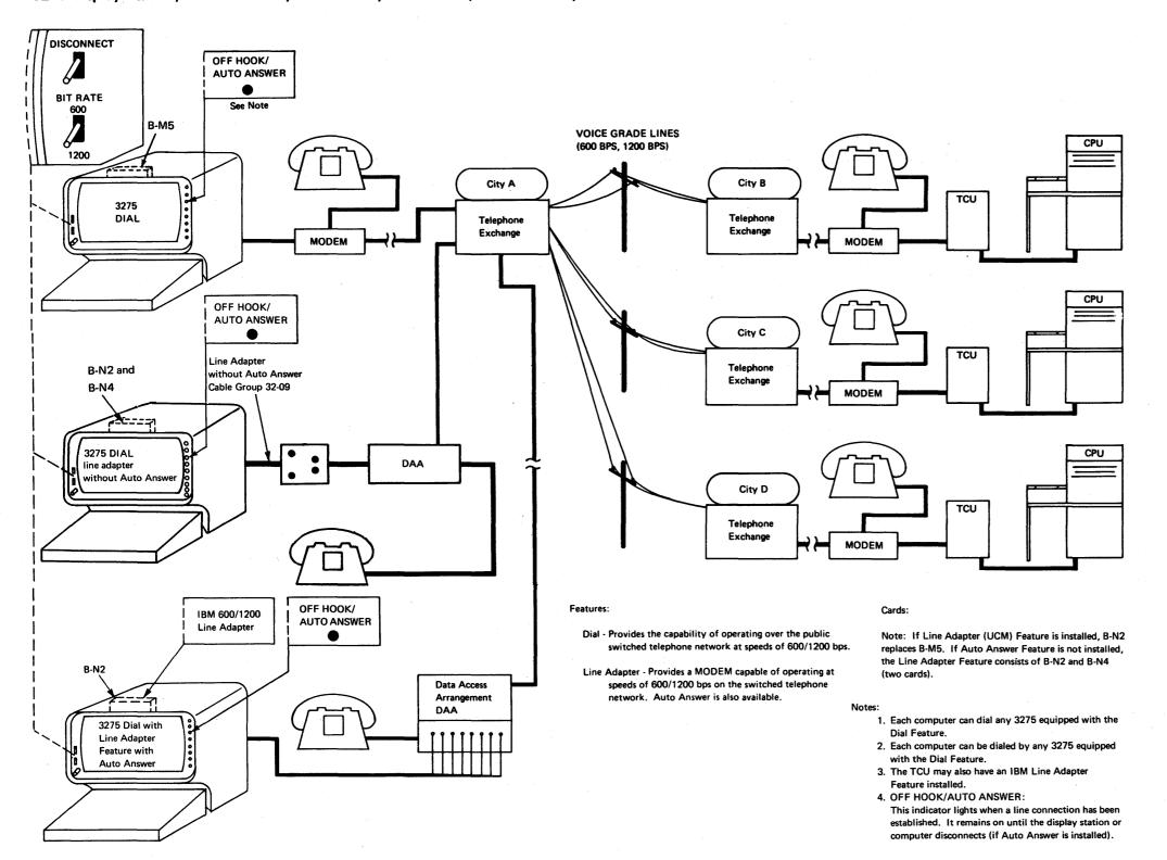
3275 Display Station, Models 1 and 2, Dial Feature, Installation (Sheet 11 of 11)
