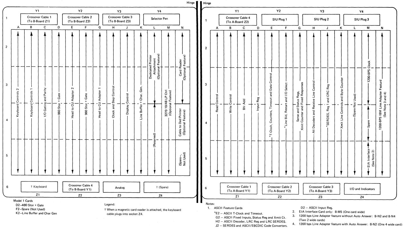
Diagram 4-13. B-Gate Card Layout by Function (Card Side)
