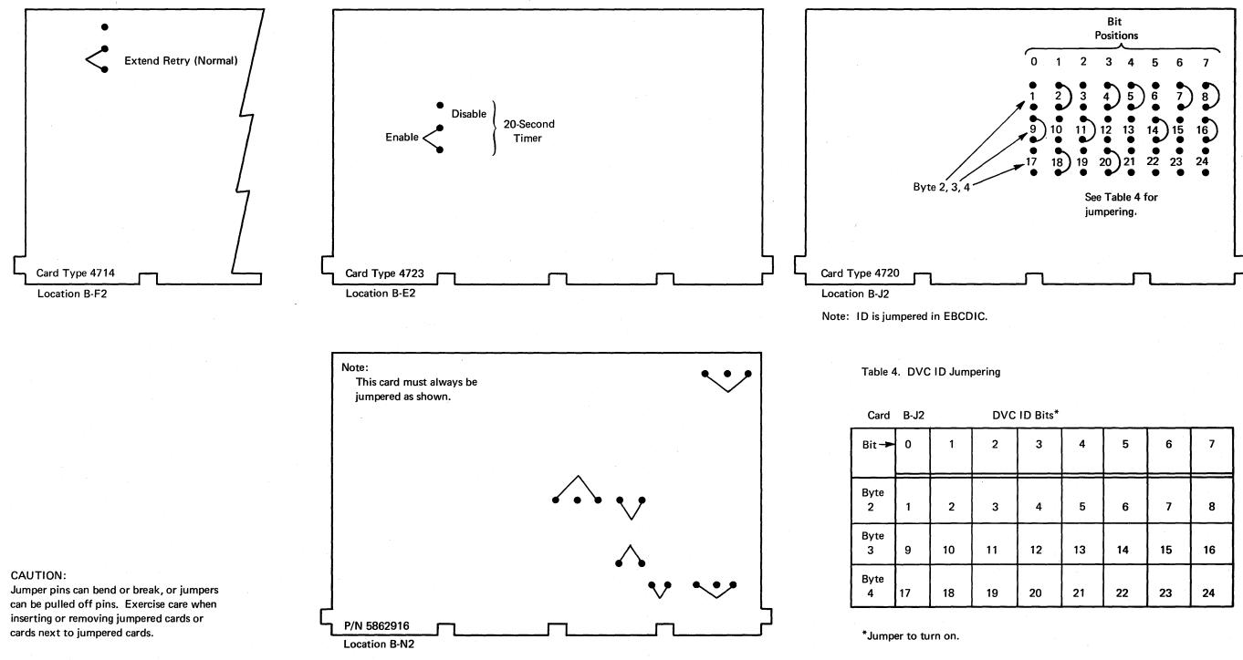
Diagram 4-11. Logic Card Jumpering – ASCII
