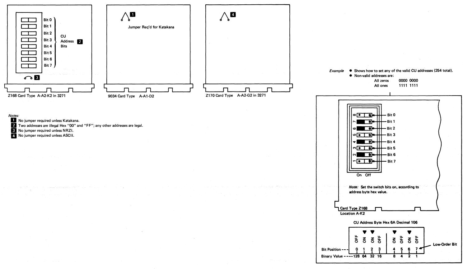
Diagram 2-6. CU Address Switch Settings and Logic Jumpering
