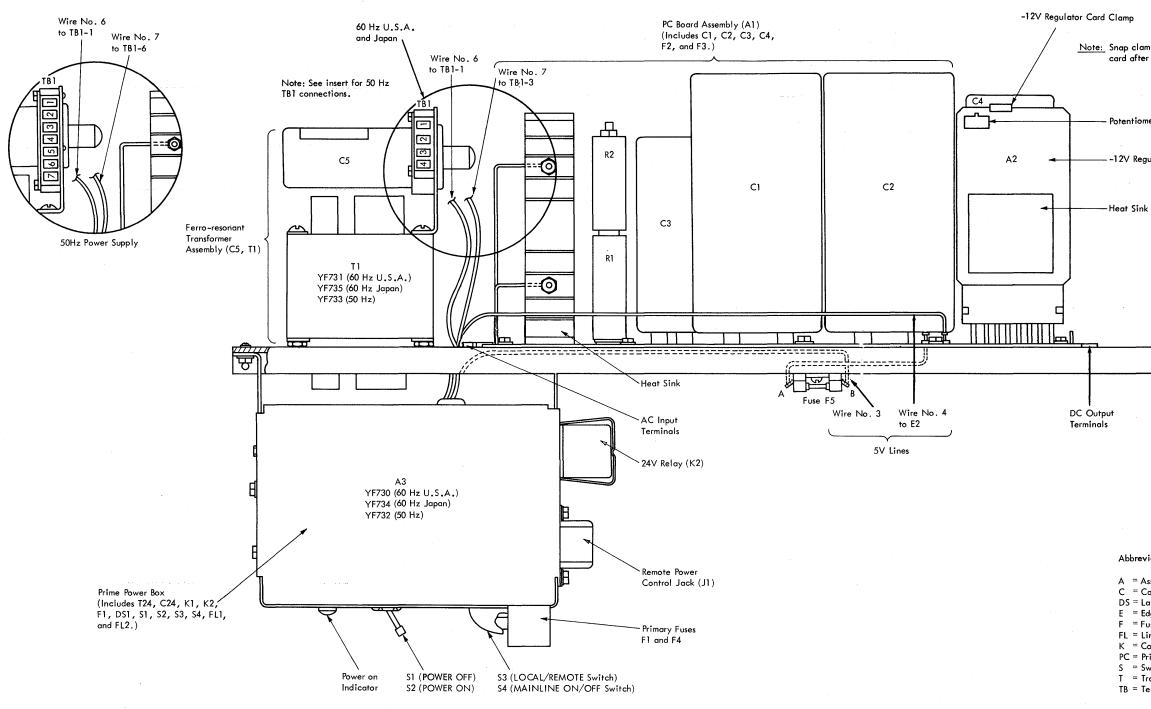
Diagram 3-5. Power Supply Component Locations (Side View)
