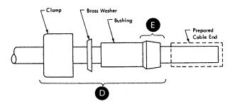
Slide the brass washer over the shield and up against the mating surface of the bushing at **F**. Wrap tape around the shield for one full turn and trim off the remaining shield strands. Install the clamp and be sure that the mating surface is tightly against the brass washer.
