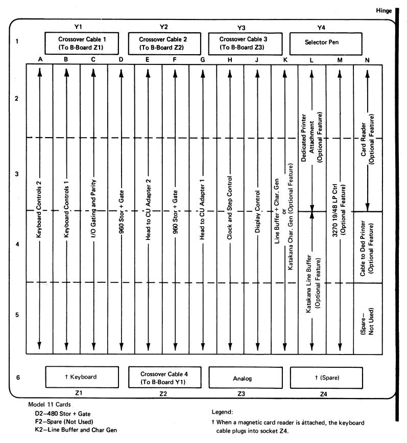
Diagram 4-18. A-Gate Card Layout by Function (Card Side)
