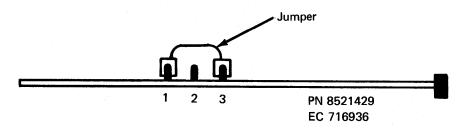
Diagram 6-12. Program Pin Jumper Connections – Motor Control Card (E2)
