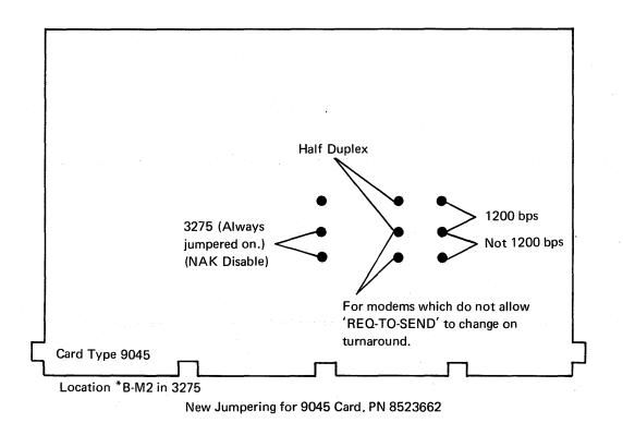
Diagram 4-5. Logic Card Jumpering – ASCII (Sheet 2 of 2)
