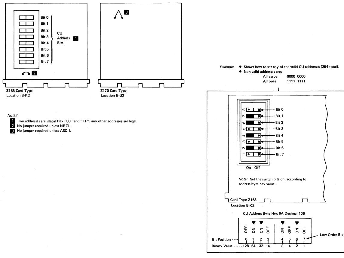
Diagram 4-19. CU Address Switches and Logic Card Jumpering
