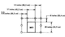
(mounted flat or in racks) Scale 1/4 inch = 1 foot
