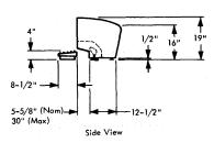
Bottom: Unit should be installed in a manner which would guarantee adequate air-flow into the underside of the unit to provide convection cooling.
