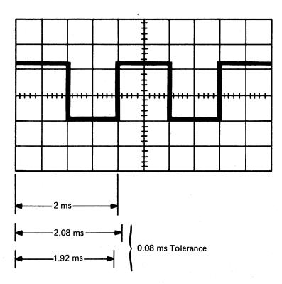
Time/Division : 0.5 Millisecond Volts/Division : 2 Volts Mode Channel : 1 Sync : Internal Coupling DC, Slope Plus Source : Internal Channel 1 Only
