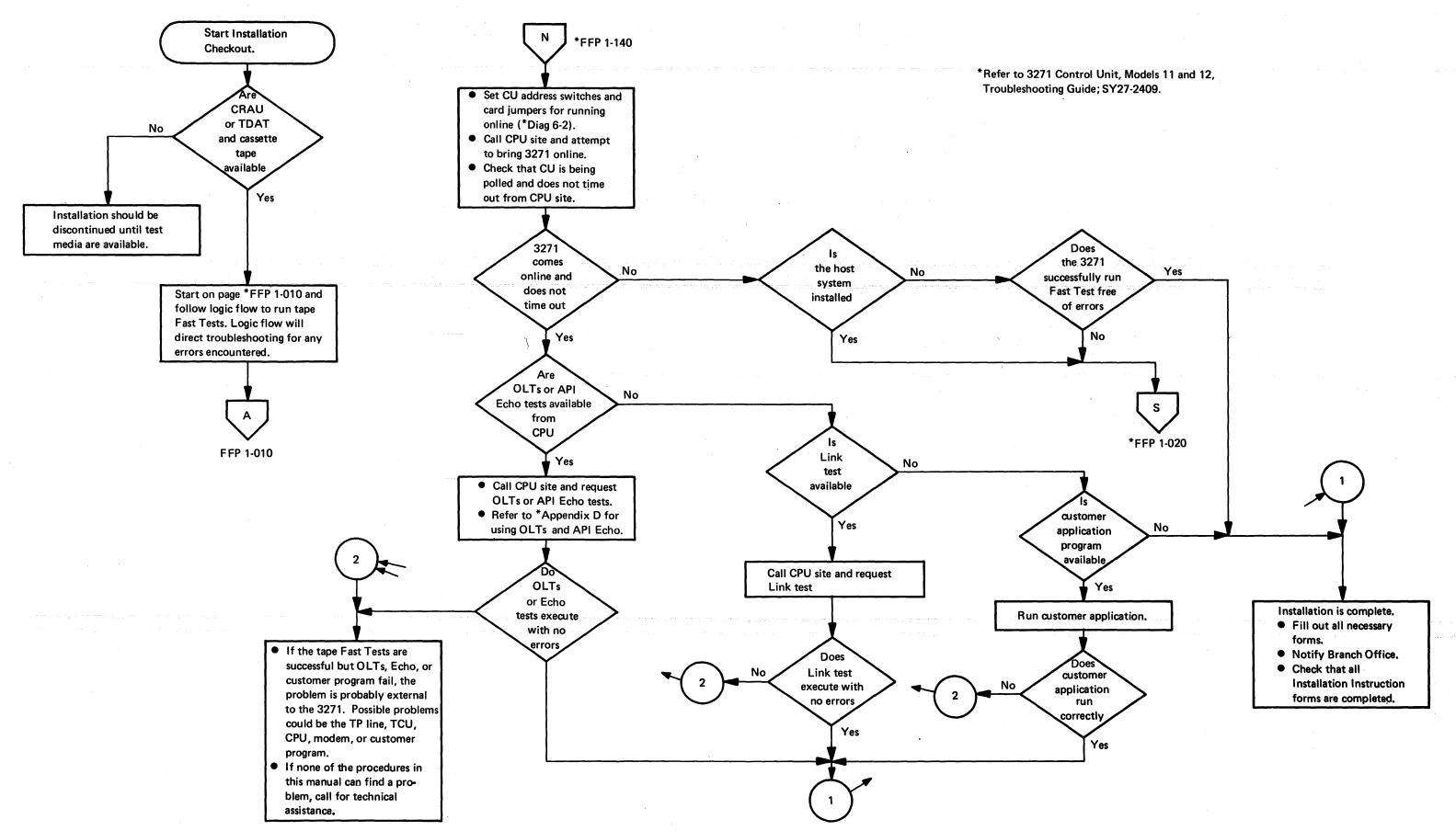
Diagram 2-5. 3271 Installation Checkout Flowchart
