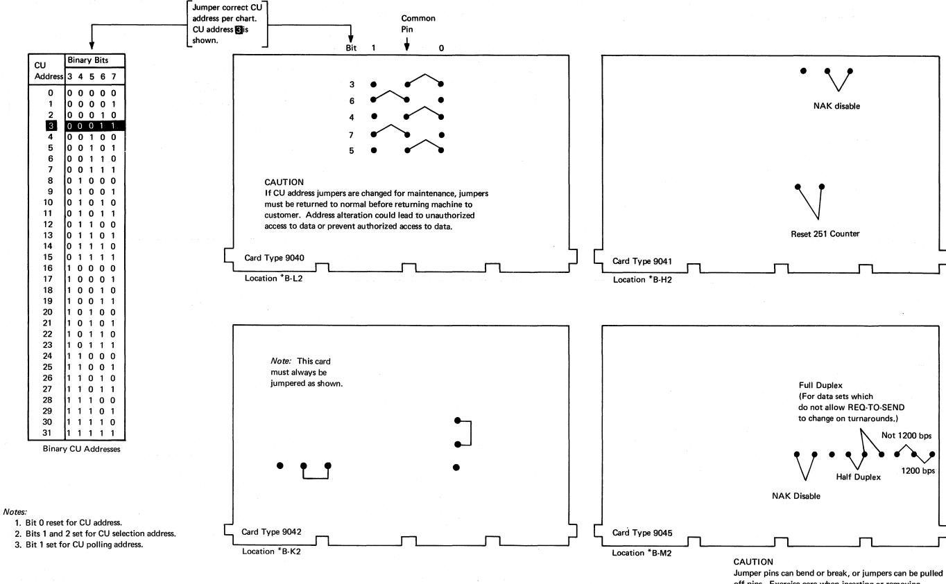
Jumper pins can bend or break, or jumpers can be pulled off pins. Exercise care when inserting or removing jumpered cards or cards next to jumpered cards.
