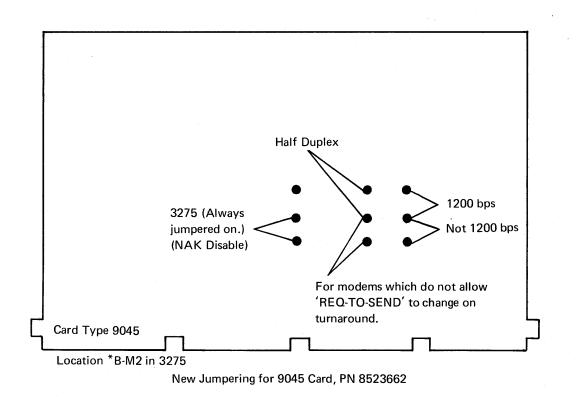
Diagram 4-4. Logic Card Jumpering – EBCDIC (Sheet 2 of 2)
