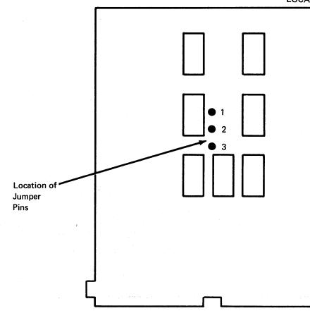
The motor control card (E2) contains most of the logic for the control of the dc stepper motor which drives the screw to run the print-head carrier in forward and reverse directions. Since the motor control card is used in both the 3284 and the 3286 printers, there is a programmable pin jumper on the card which determines whether the card will function as a 3284 stepper-motor control or a 3286 stepper-motor control. The proper programming is shown below.
