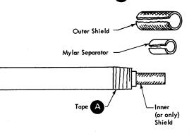
Step 3: (For two-shield cables only.) Remove Mylar separator for 1 inch (25 mm) from end for 15A-30A cables or 2-1/4 inches (57 mm) from end for 45A-60A cables. Do not cut the inner shield.
