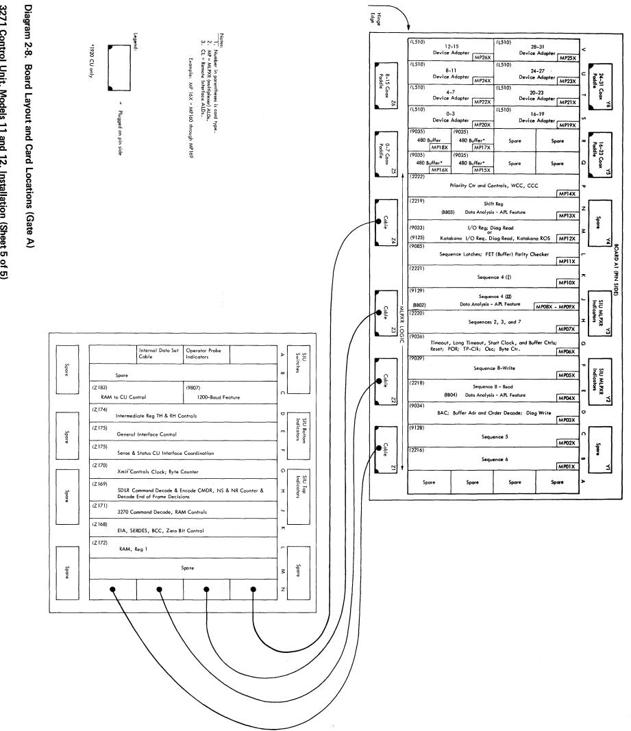
3271 Control Unit, Models 11 and 12, Installation (Sheet 5 of 5)
