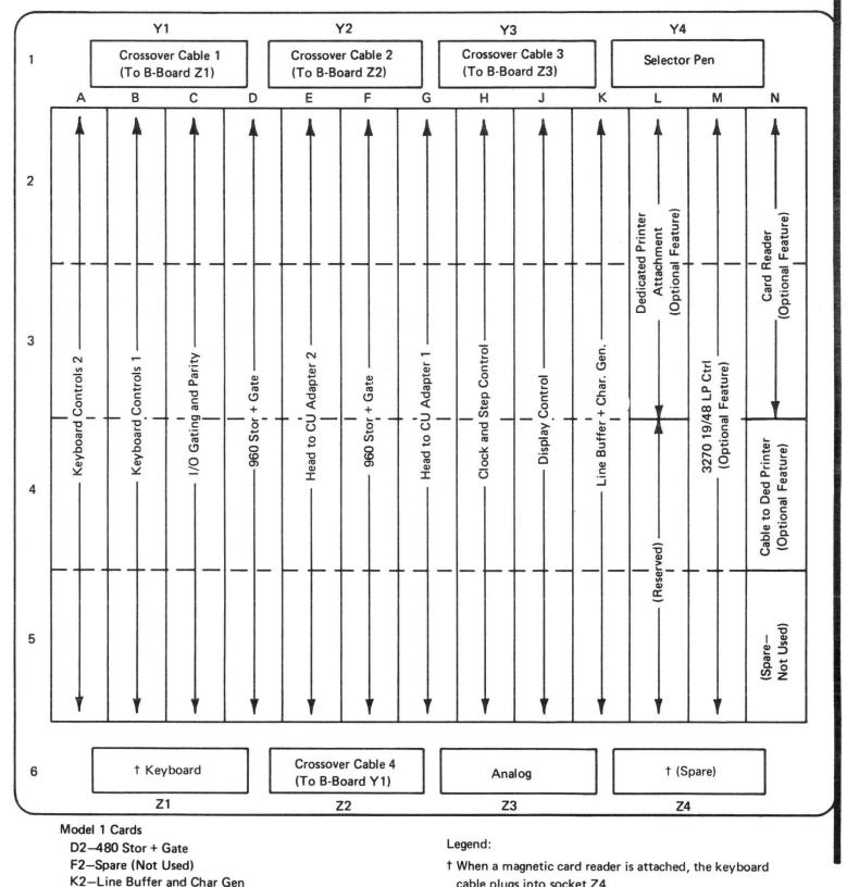
Diagram 4-2. A-Gate Card Layout by Function (Card Side)
