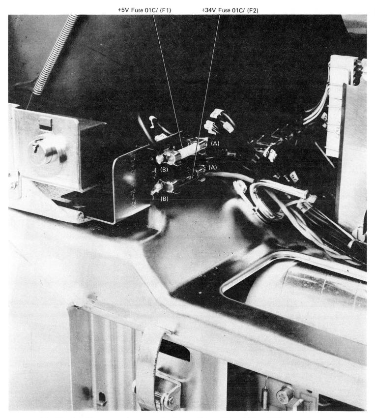
*NOTE:* This view shows the area to the right and behind the keylock, shown in Diagram 4-1, sheet 1.
