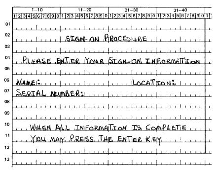
Figure 14. Sign-on Panel as Written Out on Layout Sheet
