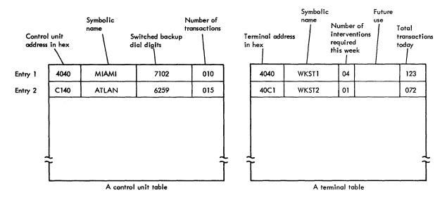
Figure 47. Table of Control Unit and Terminal Information
