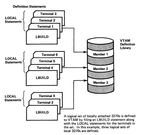
Figure 75. Grouping Locally Attached 3270s into Logical Sets
