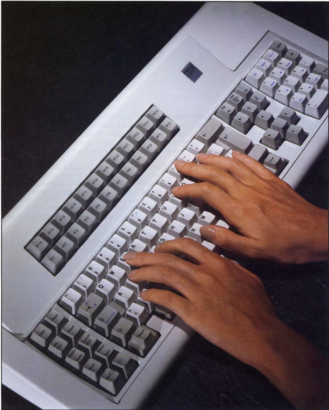
Figure 4-1. IBM 3270 Personal Computer Keyboard
