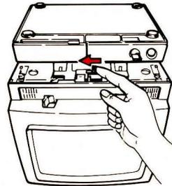
7. Remove the logic element with the stand from the video element.
