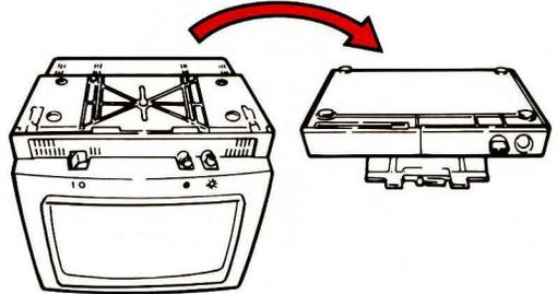
8. Move the stand to the center position on the logic element.
