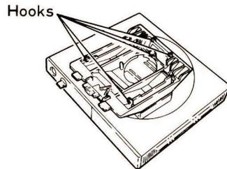
3. Insert the five hooks into the five slots of the video element.
