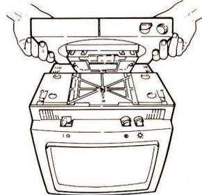
4. Holding the top edge of the front side of the video element, pull the logic element toward you until the stand snaps into place.
