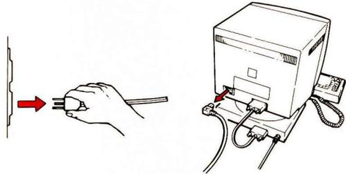
3. Unscrew and pull out **all cables** from the logic element.
