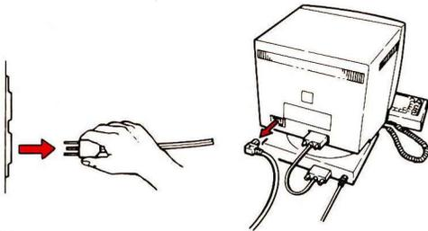
3. Unscrew and pull out all cables from the logic element.
