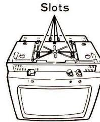
2. Locate the five hooks of the stand on the logic element.
