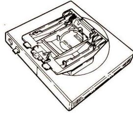
2. Lock the stand to the logic element by pinching the two gray latches on the logic element.
