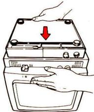
7. Make sure the logic element is locked onto the video element by moving the logic element forward and backward.
