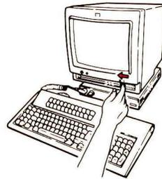
11. Insert the hollow end of the power cord into the video element and the other end into the wall outlet.
