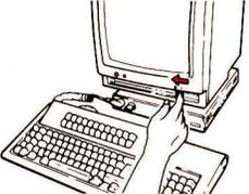
2. Unplug the keyboard cable from the logic element.
