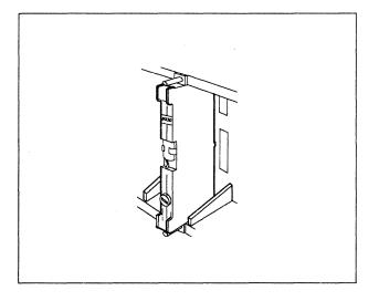
Loosen the thumbscrews in an alternating manner and remove the Encrypt/Decrypt Adapter by pulling it straight out.
