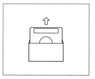
With the label facing to the left, insert the Utility diskette into Diskette Drive 1 and close the lever.
