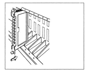
Tighten the thumbscrews in an alternating manner. For example, tighten one screw two turns and then the other two turns until both screws are tightened completely.
