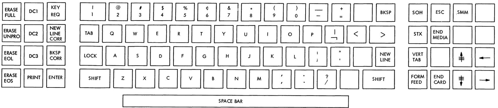
Figure 2772-11. USASCII Keyboard for Printer and Display
