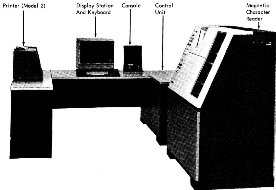
IBM 2770 Data Communication System: Three Typical Configurations
