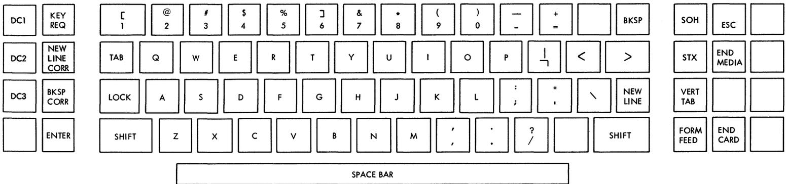
Figure 2772-10. EBCDIC Keyboard for Printer and Display
