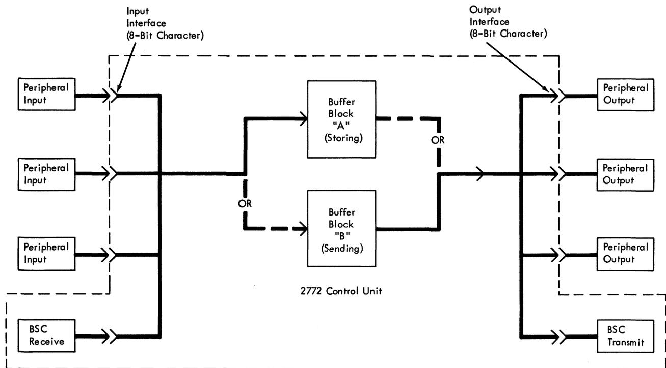
Figure 2772-1. Schematic of 2772 in a 2770 System
