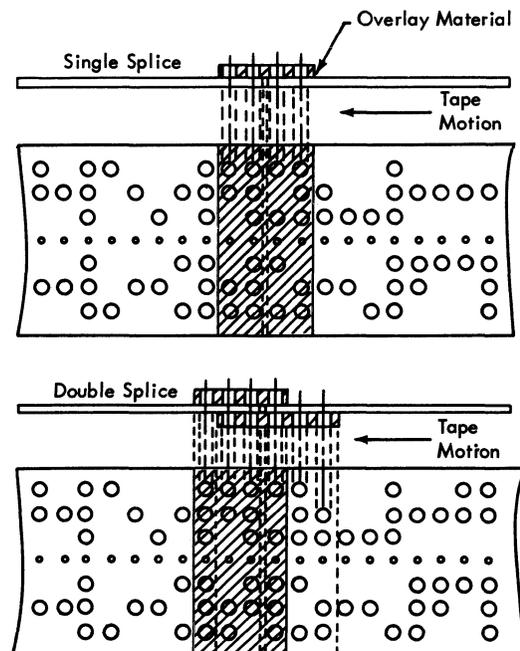
Figure PT-2. Butt-Joint Splice
