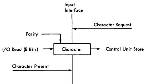
Note: Timing determines which interface signal is the demand and which is the response.
