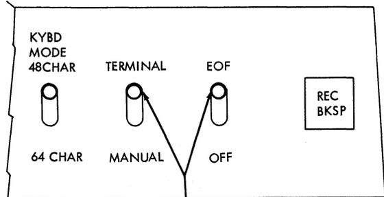
These switches are added when 2772 attachment feature is installed.
