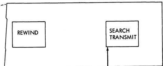
This key is changed from SEARCH to SEARCH/TRANSMIT when 2772 attachment feature is installed.
