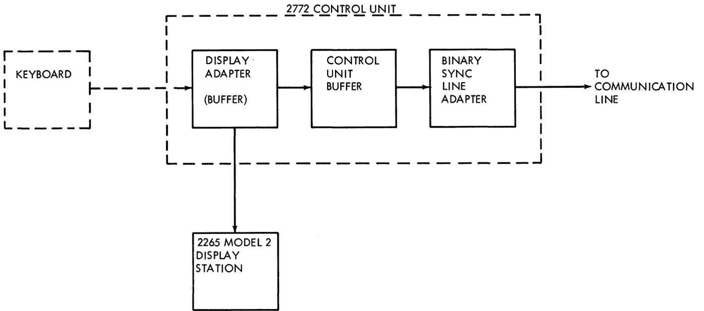
Figure 2265-2. Transmit Operation in Line Mode
