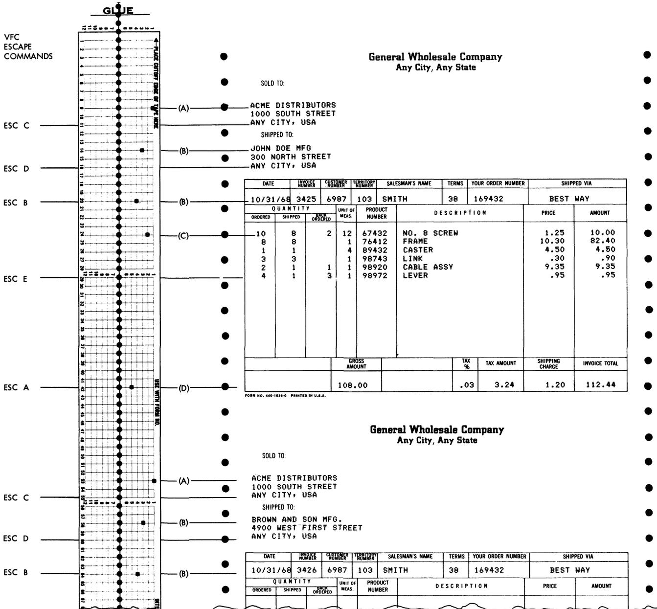
Figure 2213-7. Tape-Form Correlation for a Typical Application
