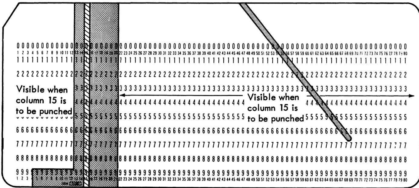
Figure 545-6. Card Visibility at the Punch Station
