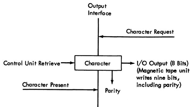
Note: Timing determines which interface signal is the demand and which is the response.
