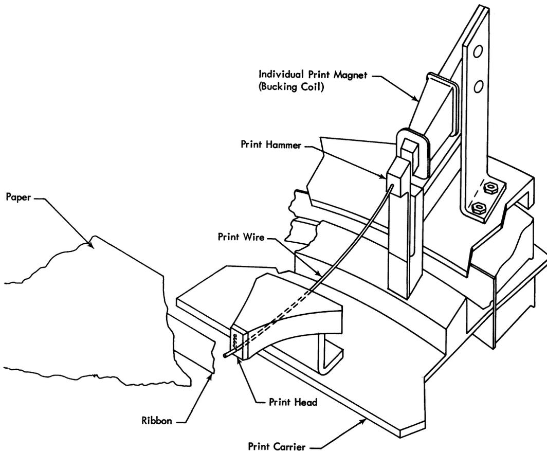
Figure 2213-2. Print Mechanism
