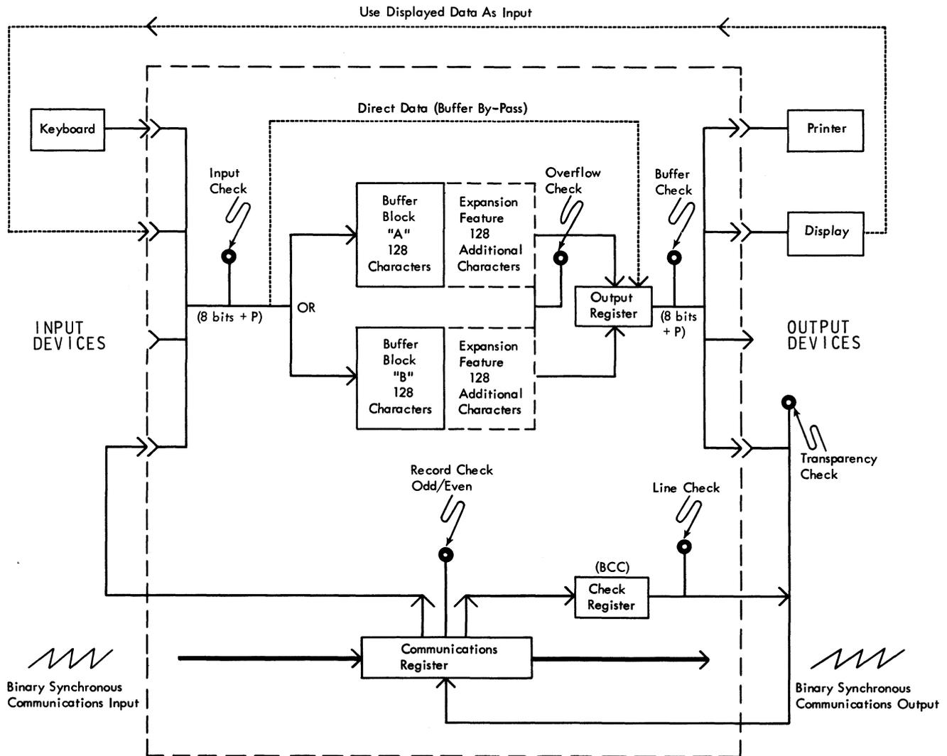
Figure 2772-3. 2772 Data Flow and Check Points
