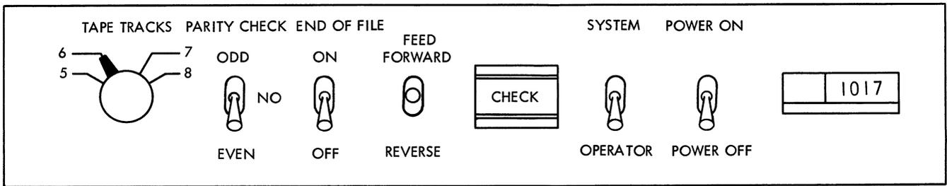
Figure 1017-2. IBM 1017 Operator Controls(Reader)
