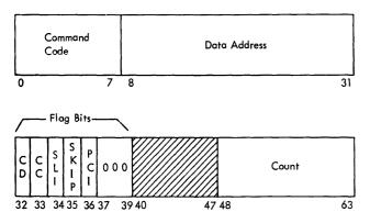
A complete discussion of each of the fields within a channel-command word (CCW) is included in the publication, <u>IBM System/360</u>, <u>Principles of</u> <u>Operation</u>, Form A22-6821.
