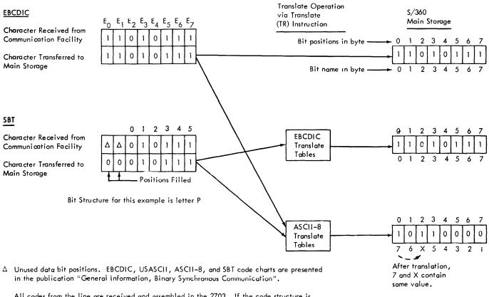
All codes from the line are received and assembled in the 2703. If the code structure is fewer than eight data bits, it is right justified and transferred to its byte location in main storage. Any missing bit positions in the main storage byte are filled. If the code received from the line has an 8-bit structure, it is transferred directly to its main storage byte location as in above examples.
