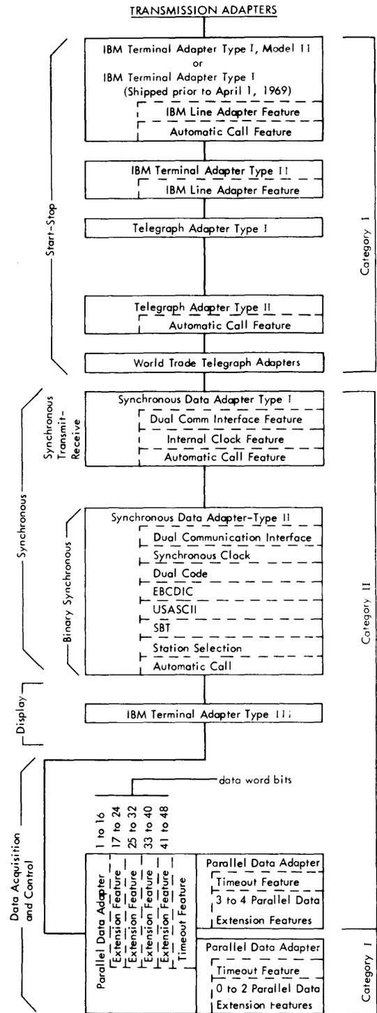
Figure 4. Physical Size Categories of 2701 Transmission Adapters and Adapter Features
