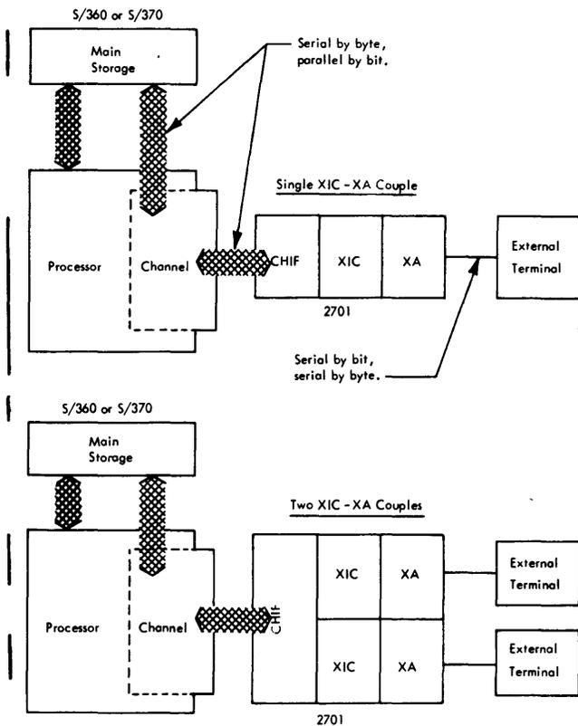
Figure 2. Functional Sections Illustrating Relationship of 2701 to System/360 or System/370, and External I/O Devices (Terminals)
