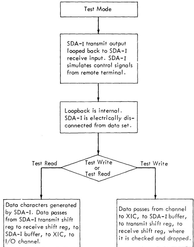
Figure 53. Test Read and Test Write--SDA-I Operation
