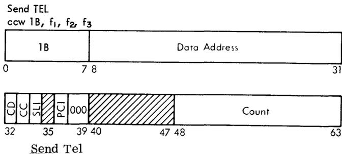
For the Send Tel command to be accepted, the SDA-I must be in the operational mode. The program issues this command to cause the SDA-I to transmit a Tel signal to the remote terminal. The remote terminal should automatically respond with a Tel signal. The Send Tel command ends normally with Channel End and Device End when the Tel response is received.
