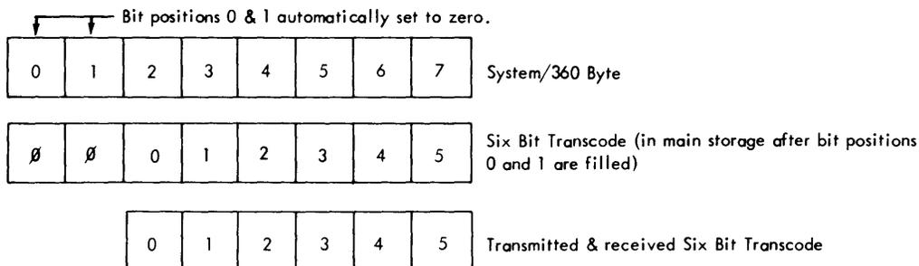
Figure 58. Six-Bit Transcode (as used in Binary Synchronous Communication)
