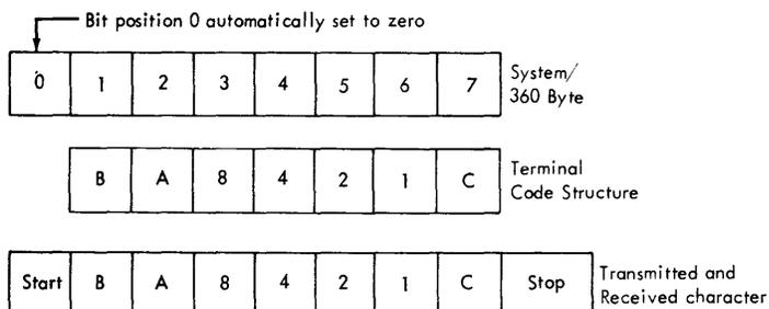
On receive operations, the start-stop bits are deleted at the 2701.
