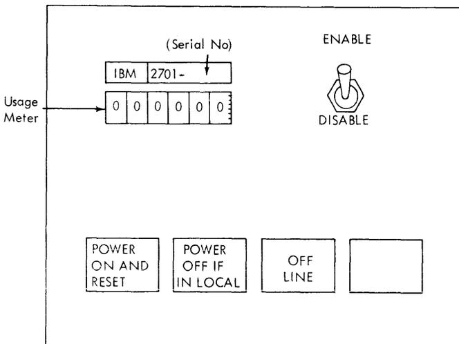
Figure 9. Operator's Control Panel--IBM 2701
