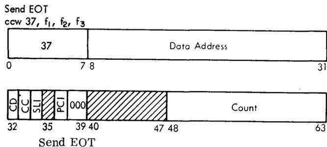
For the Send EOT command to be accepted, the SDA-I must be in the operational mode. The program issues this command to cause the SDA-I to transmit the end-of-transmission (EOT) control signal to the remote terminal. The Send EOT command ends with Channel End and Device End when the EOT response is received. When the Inq response is received, the command ends with Channel End, Device End, and Unit Check status with the Inquiry sense bit set to one.
