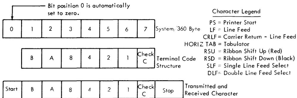
On receive operations, the start-stop bits are deleted at the 2701.
