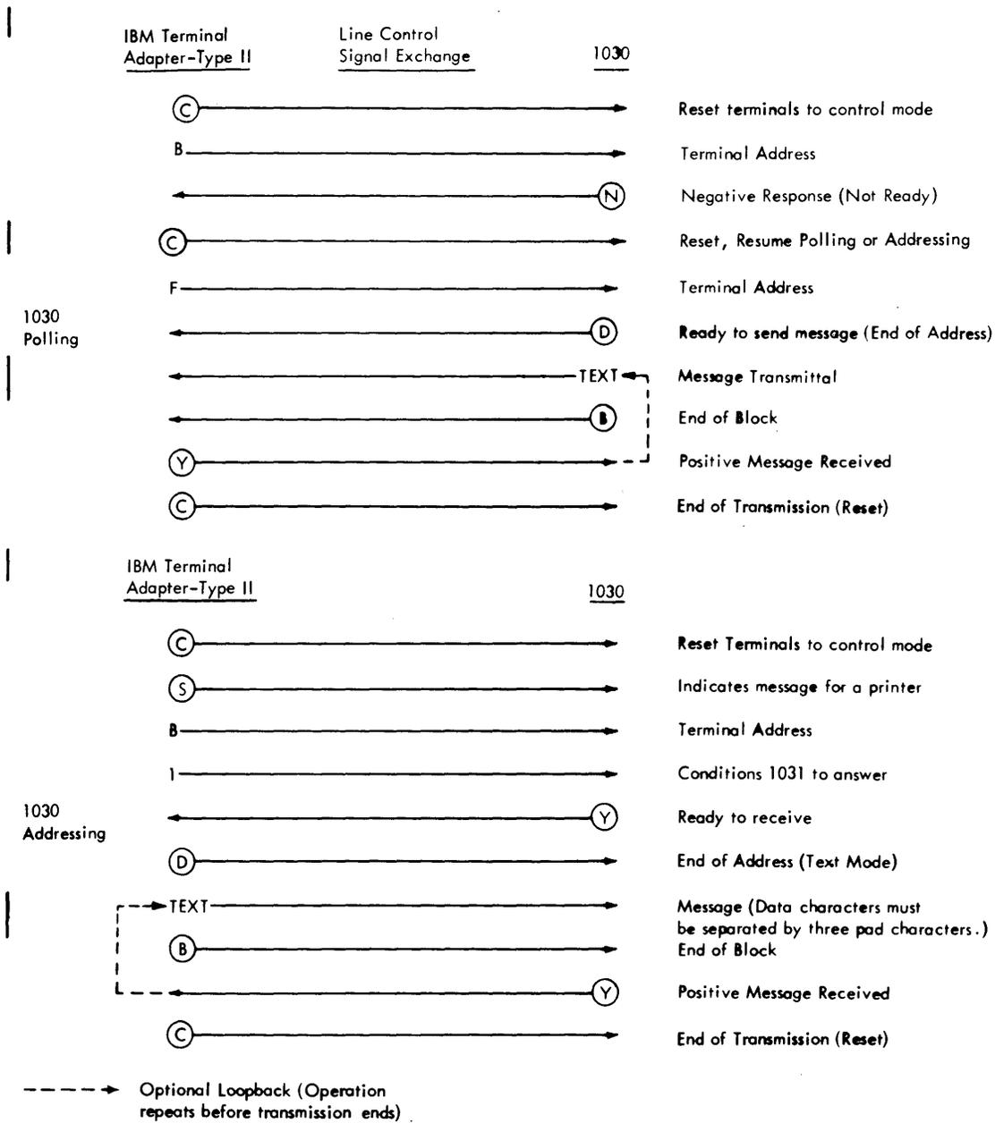
Figure 28. IBM Terminal Adapter Type II and IBM 1030 Line Control Sequences
