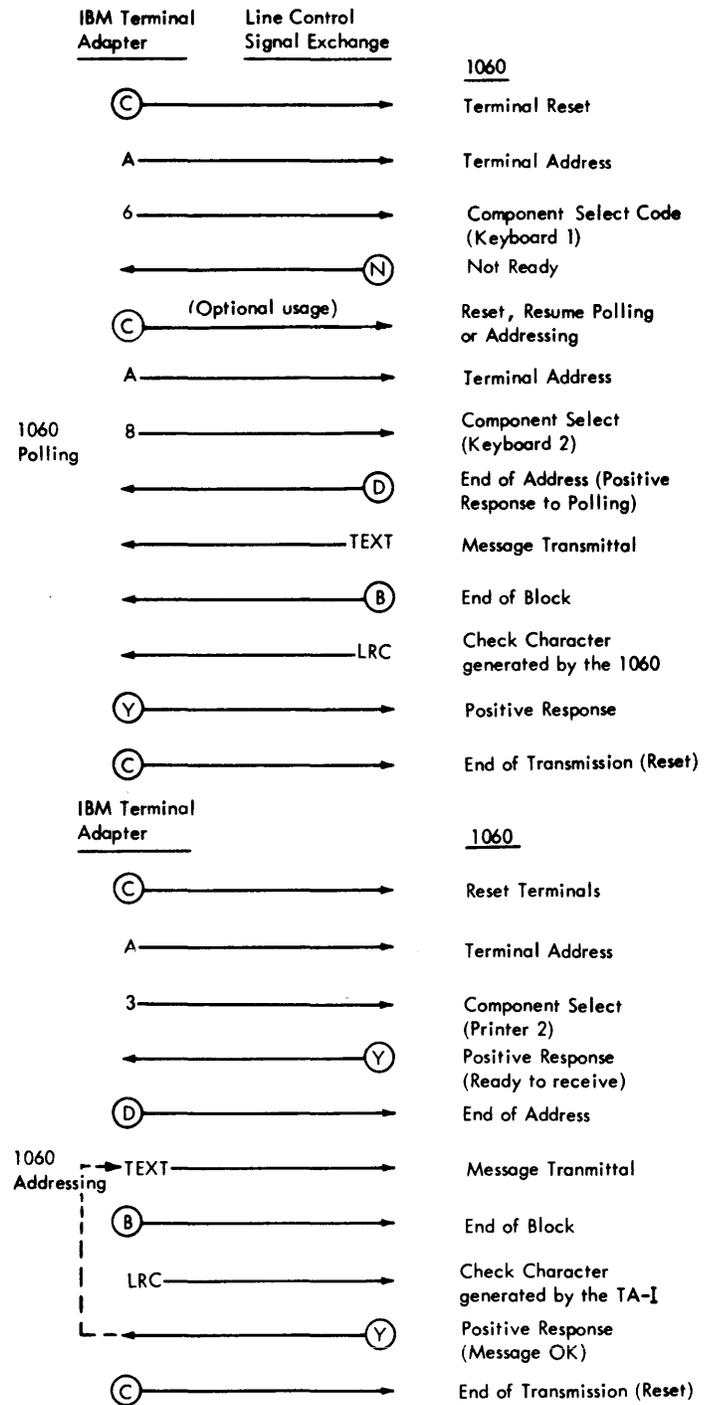
Figure 21. Line Control Sequences--IBM Terminal Adapter Type I with IBM 1060
