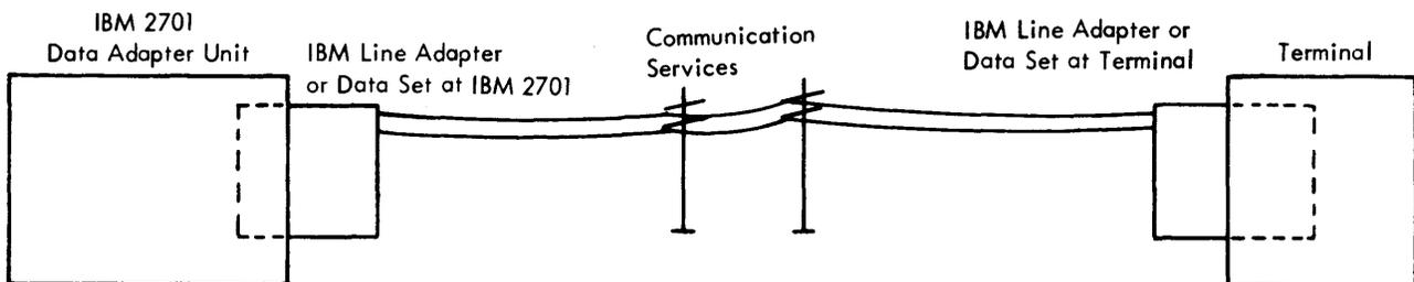
Figure 10. Terminal Connection via IBM Line Adapters or Data Sets and Communications Services
