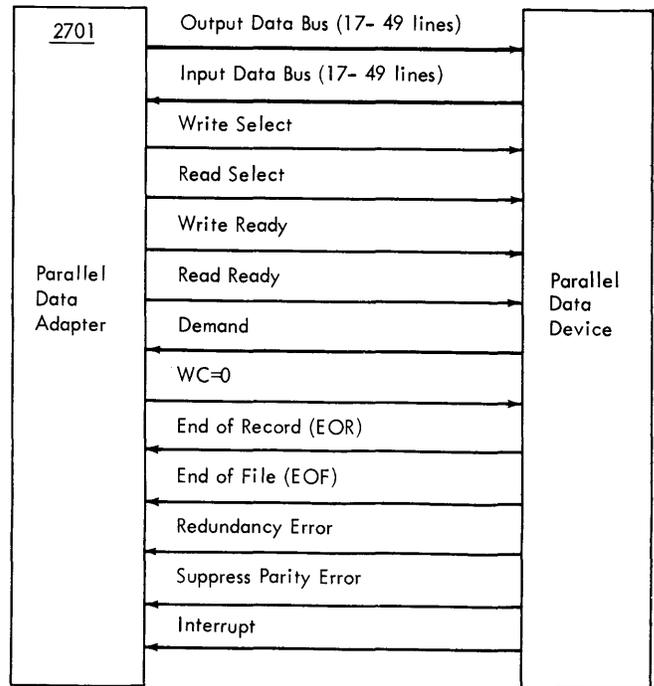
Figure 38. Parallel Data Adapter Interface
