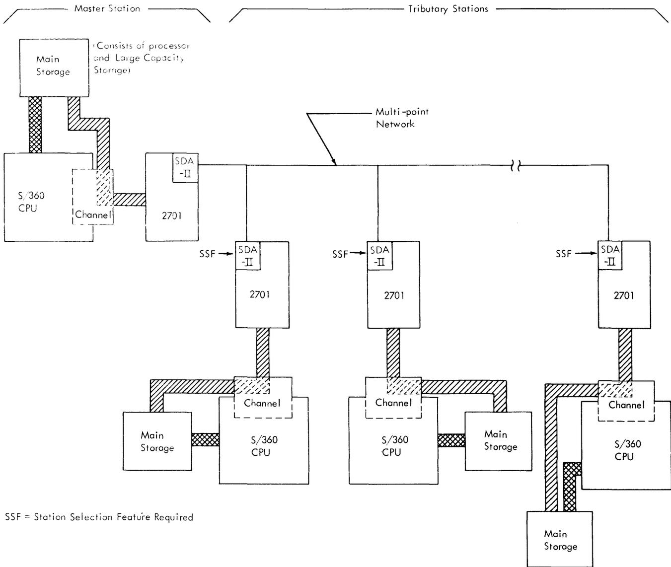
Figure 55. SDA-II in Multi-Station Operation
