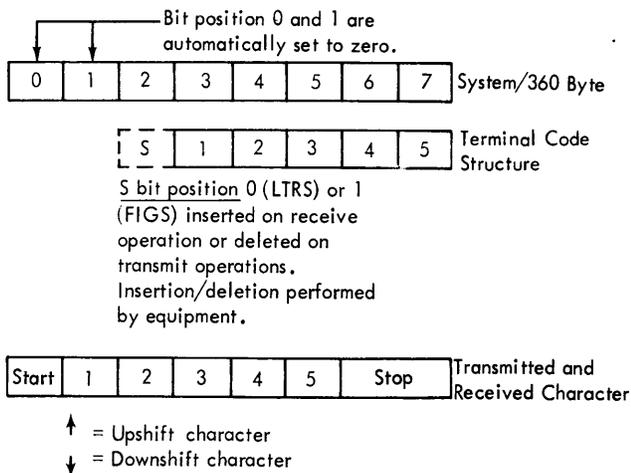
Figure 32. Code Structure for AT&T 83B2/83B3 and Western Union Plan 115A Terminal--System/360 Oriented
