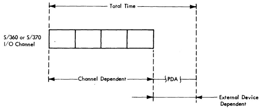
Note: This concept applies to all sizes (16-bit-word thru 48-bit-word) of the 2701 Parallel Data Adapter.
