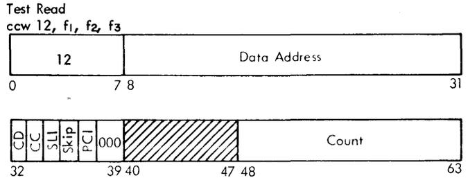
Test Read. For the Test Read command to be accepted, the SDA-I must be in the operational mode, and must have been placed in the test mode by a Set Mode command. As in the case of Test Write, the SDA-I transmit-section output is looped back to the SDA-I receive-section input.
