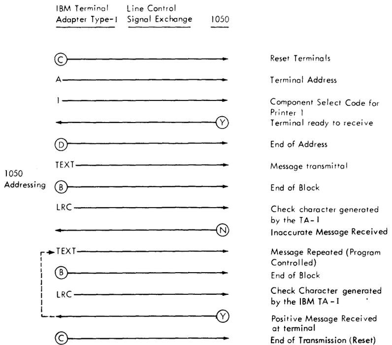
Figure 20. Line Control Sequences--IBM Terminal Adapter Type I with IBM 1050
