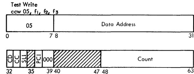
Test Write. For the Test Write command to be accepted, the SDA-I must be in the operational mode, and must have been placed in the test mode by a Set Mode command. Test Write operates similar to Write, with the following exceptions:
