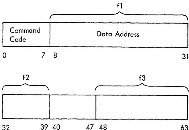
Figure 12. Commands for Start/Stop Adapters
