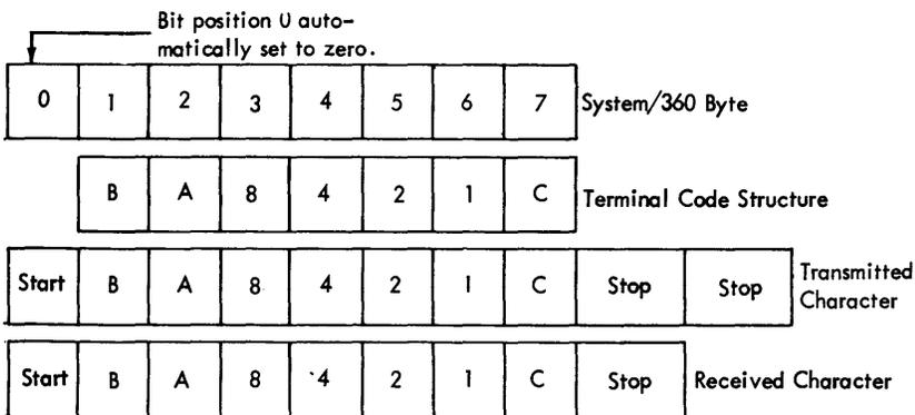
On receive operations, start-stop bits are deleted by 2701.
