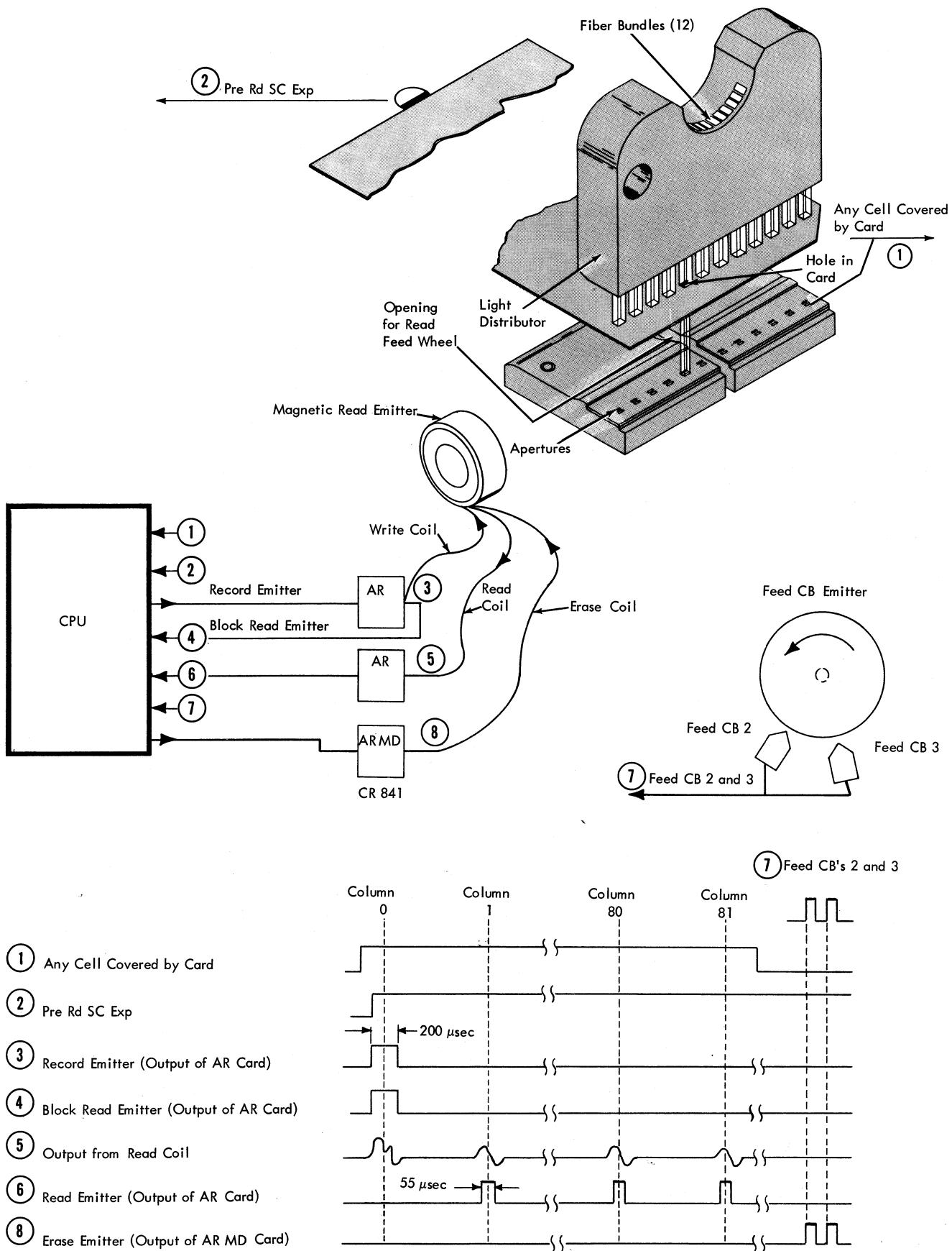
Figure 2-9. Electrical Operation of Magnetic Read Emitter
