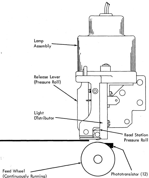
Figure 2-6. Operation of Read Unit
