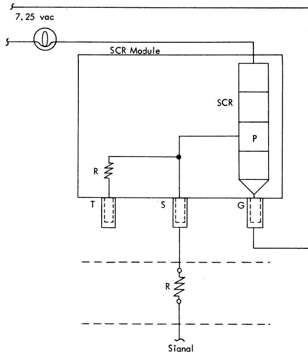
Figure B-1. Indicator Lamp Power Module
