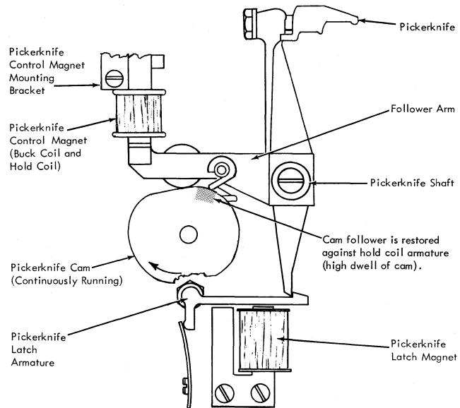
Figure 2-4. Operation of Pickerknife Control Magnet and Latch
