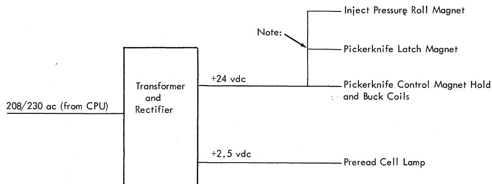
Note: This line supplies +24 volts to the logics for the components connected to the line.
