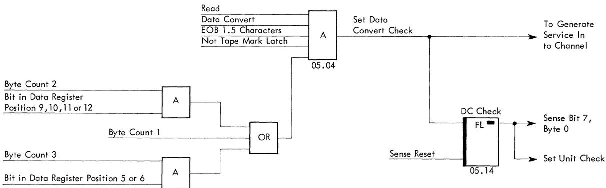
FIGURE 4-5. DATA CONVERT CHECK (DCC)
