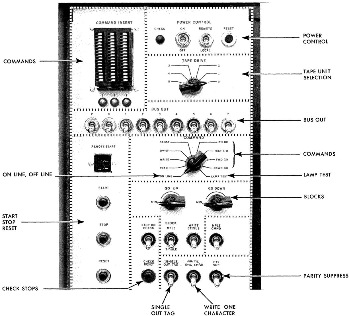
FIGURE 6-2. FUNCTIONAL GROUPING OF CE PANEL CONTROLS
