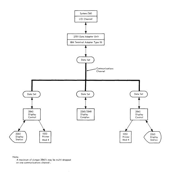
Figure 1. Typical Connection of an IBM 2845 Display Control to a Remote Central Processor Showing Application in a Multidrop Communications Network.
