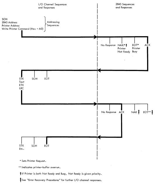
Figure 12. Write Printer, Sequence/Response Diagram
