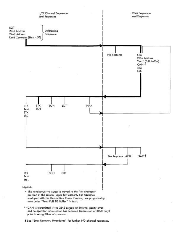
Figure 9. Read Addressed Full DS Buffer, Sequence/Response Diagram
