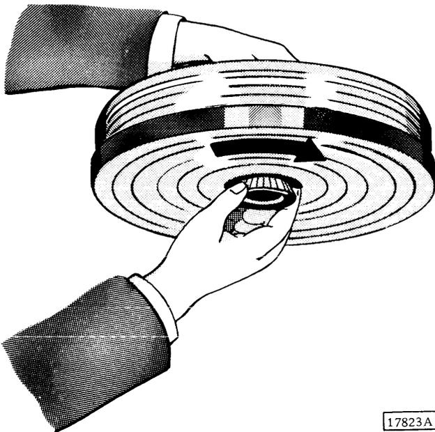
5. Lift cover containing disk pack from spindle.
