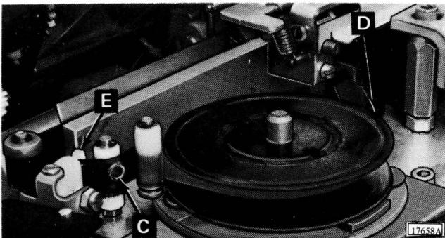
7. Verify that leading end of ribbon is firmly hooked onto empty spool and metal eyelet (C) on ribbon is somewhere between spool (D) and ribbon reversing mechanism (E).
