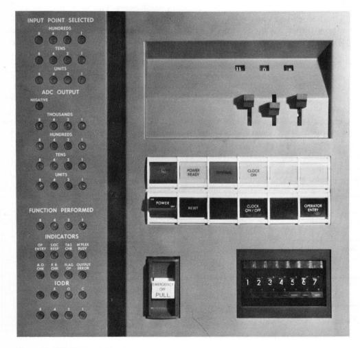
Figure 33. 1711 Operator's Panel
