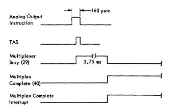
Figure 31. Analog Output Interrupt Timing
