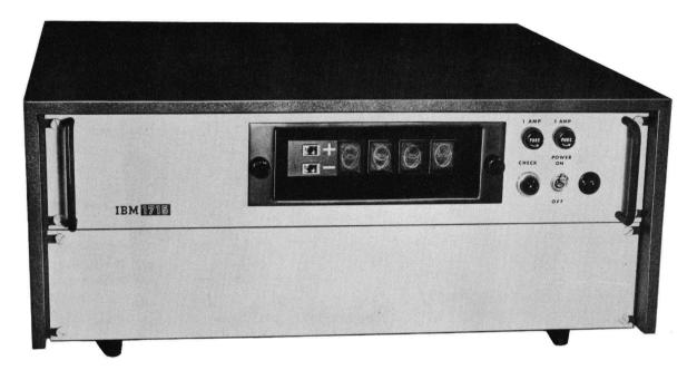
Figure 24. IBM 1715 Digital Display Unit
