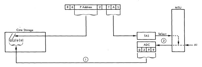
Figure 29. Select ADC Register Instruction Data Flow
