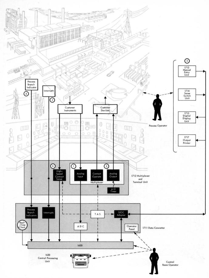
Figure 4. Data Flow Diagram of 1710 Control System
