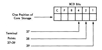
The corresponding bit is stored if a contact is closed; the bit position is blank if the contact is open. For example, if the first and third contacts are closed, the core storage position assigned to the group of three contacts contains a 4 bit and a 1 bit. Table 6 illustrates this by showing the bit configuration for all possible combinations of the three contacts when open and
