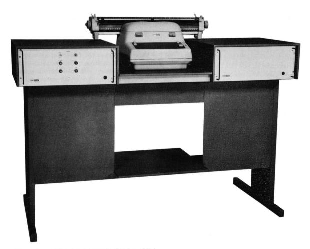
Figure 25. IBM 1717 Output Printer with 1716 Control Units
