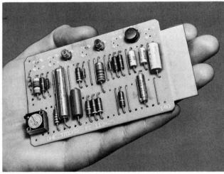
Figure 2. IBM SMS Card
