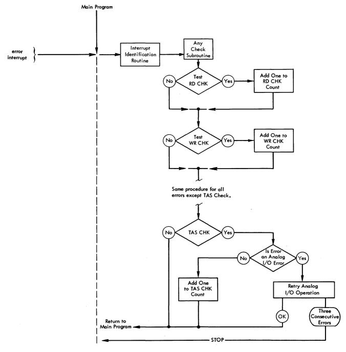
Figure 18. Error Analysis Subroutine Logic
