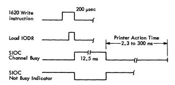
Figure 26. Output Printer Timing
