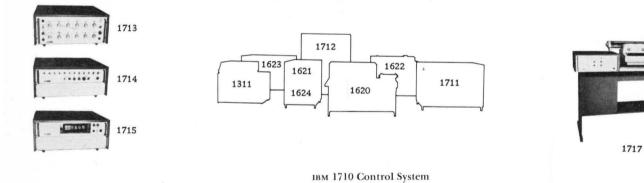
The IBM 1710 Control System is specially designed for controlling processes in such industries as petroleum refining, chemical processing, electric utility, natural gas transmission, and steel production. It is an on-line control system that meets the requirements demanded by industrial processing management by offering versatility of operation, reliability, and ease of expansion through modular construction of the System.
