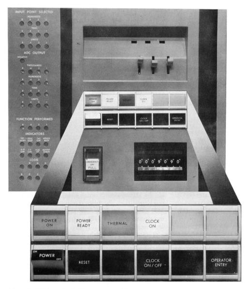
Figure 34. 1711 Operating Switches, Keys, and Lights
