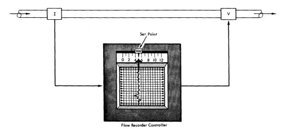
Figure 12. Automatic Control Loop
