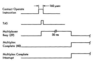
Figure 32. Contact Operate Interrupt Timing
