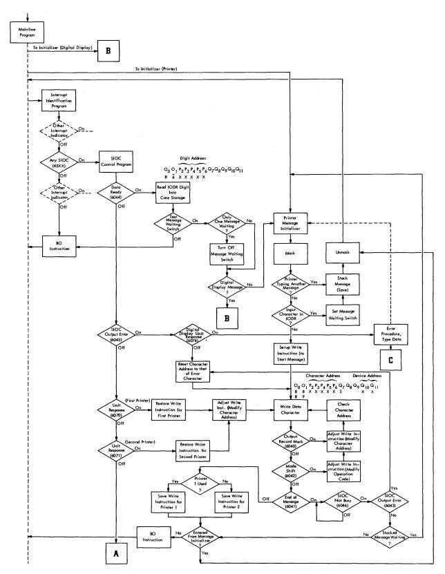
Figure 27a. Block Diagram for stoc Program, Part 1
