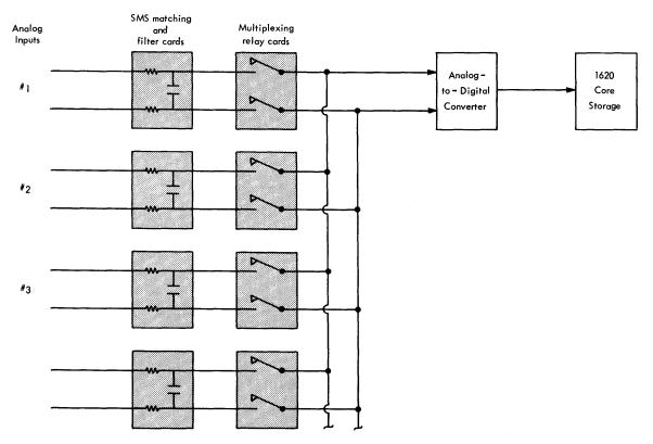
Figure 6. Analog Input Data Flow
