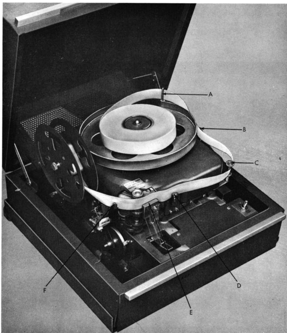
Figure 3. IBM Tape Punch
