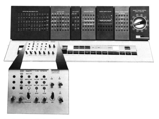
Figure 22. Indicators and Switches on 1620 Console
