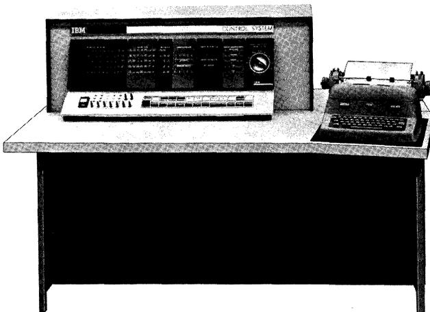
Figure 1. IBM 1620 Model 1 Central Processing Unit
