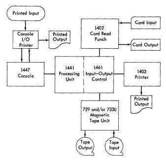
Figure 22. Tape-Oriented 1460 System Schematic
