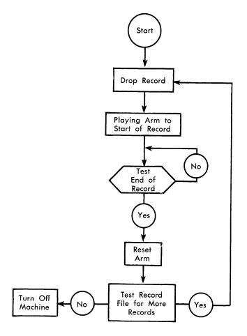
Figure 2. Block Diagram of a Program
