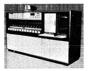
Figure 36. IBM 1418 Optical Character Reader, Model 2
