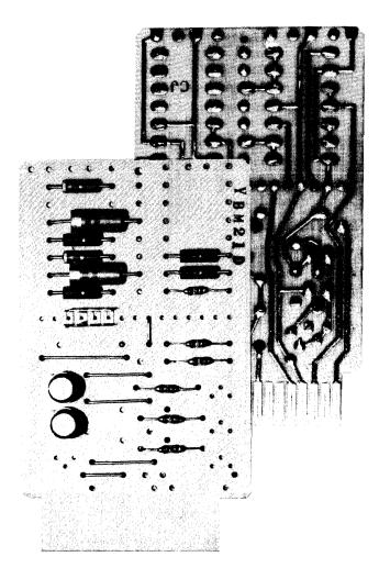
Figure 6. Transistor Cards
