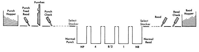
Figure 31. Punch-Feed-Read Schematic
