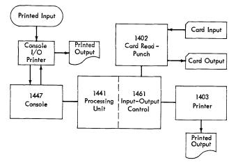
Figure 8. Card-Oriented 1460 System Schematic
