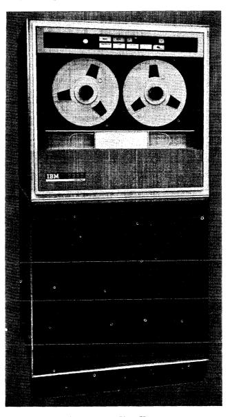
Figure 24. IBM 7330 Magnetic Tape Unit
