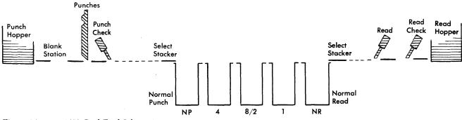
Figure 14. IBM 1402 Card-Feed Schematic
