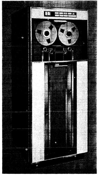
Figure 23. IBM 729 Magnetic Tape Unit
