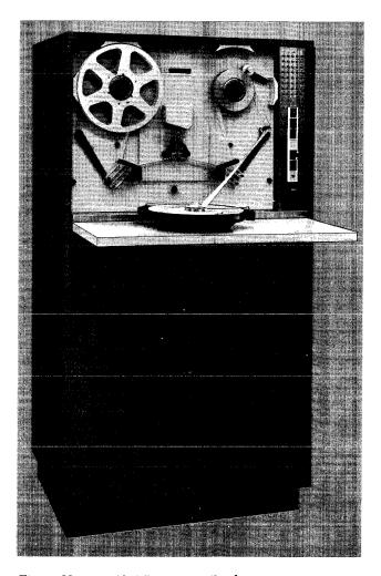
Figure 33. IBM 1011 Paper Tape Reader
