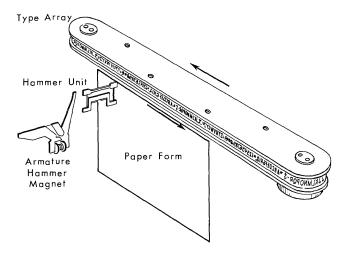
Figure 17. Schematic of Printing Mechanism
