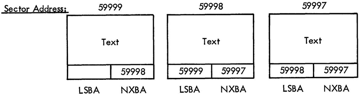
Figure 4. Working storage with two-way chaining
