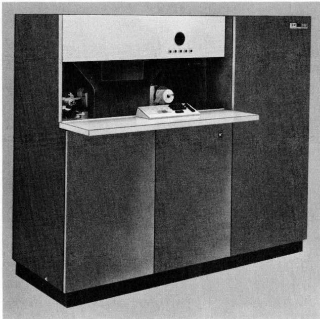
Figure G-58. IBM 1285 Optical Reader
