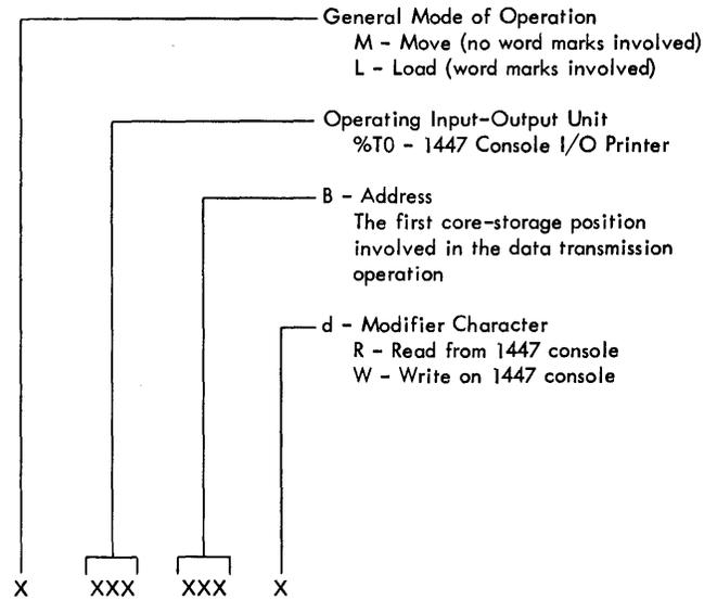
Figure 61. 1447 Console I/O Printer Instruction Format
