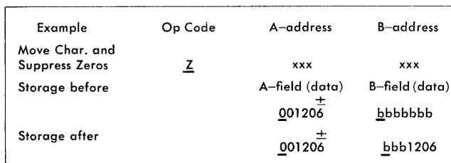
Figure 38. Move Characters and Suppress Zeros Operation Example
