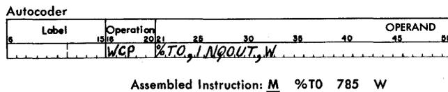
Figure 63. Write on 1447 Console
