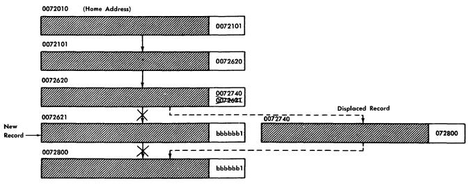
Figure 6. Additions to a Disk-Storage Chain
