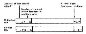
Figure 12. Dummy Record Preceding Additions Area
