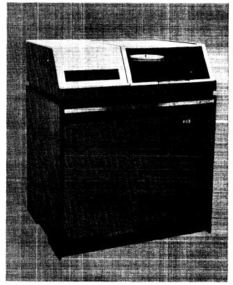
Figure G-15. IBM 1311 Disk Storage Drive
