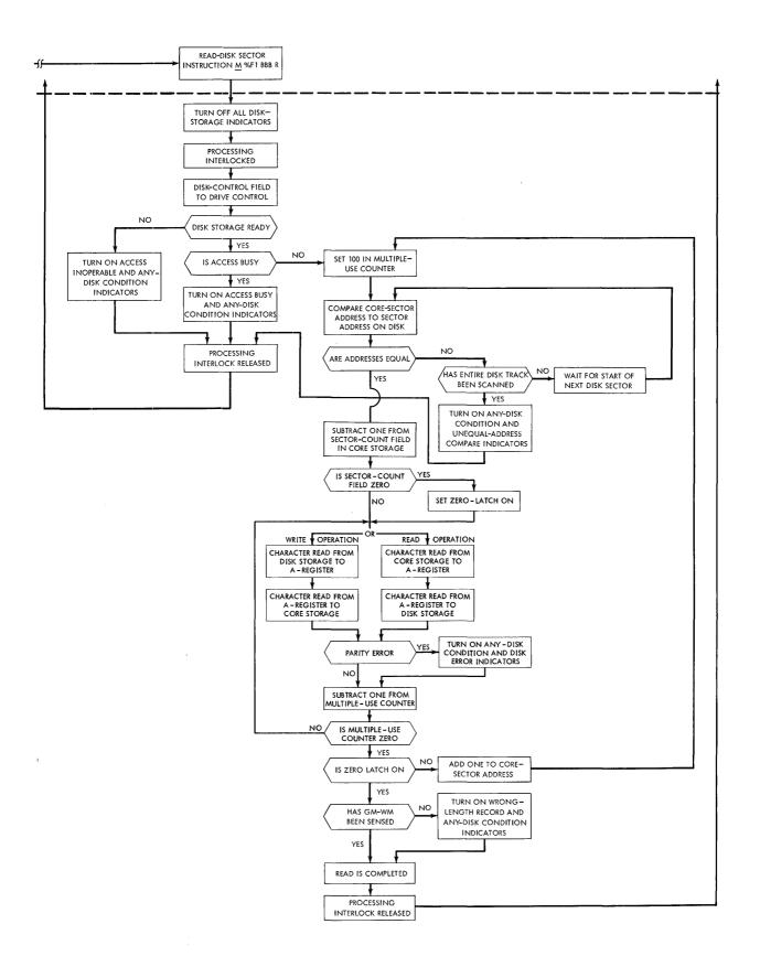
Figure G-19. Read/Write Disk Functional Schematic
