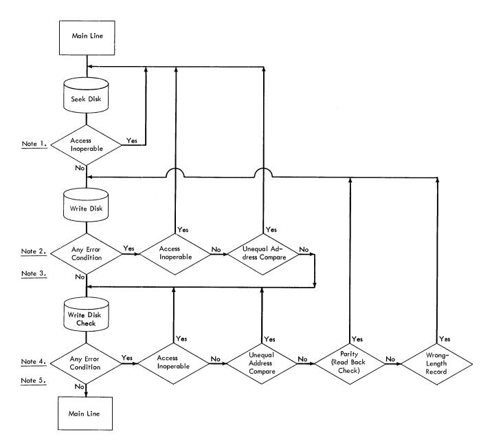
Figure G-14. IBM 1405 Disk Write Error Routine
