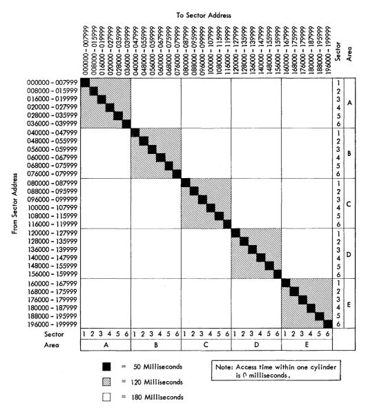
Figure G-55. Sector-Address-to-Sector-Address Access Time
