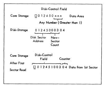
Figure G-42. Read Disk - Sector-Count Overlay Operation
