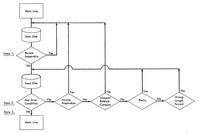
Figure G-13. IBM 1405 Disk Read Error Routine
