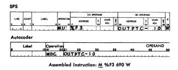
Figure G-28. Write Disk Check
