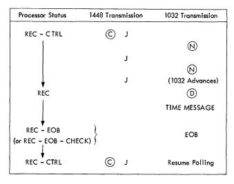
Figure 30. Point-to-Point Operation (1032 to Processing Unit -1448)
