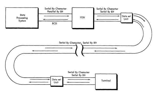
Figure 6. Data Flow Between Processing Unit and Terminals
