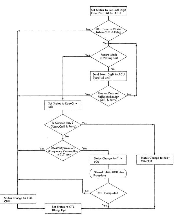
Figure 28. Automatic Calling Procedure
