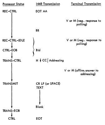
Figure 32. Processing Unit-1448 to Telegraph Terminal
