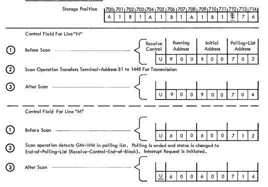
Figure 11. Scan Operation and Control Field During Polling
