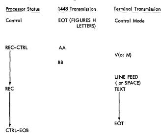
Figure 31. Telegraph Terminal to Processing Unit-1448
