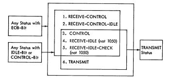
Figure 21. Processing Unit Line-Status Character Transistions
