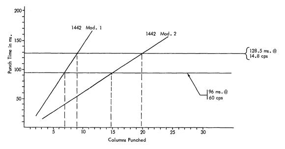
Figure 24. Punch Time vs. Columns Punched (1442)
