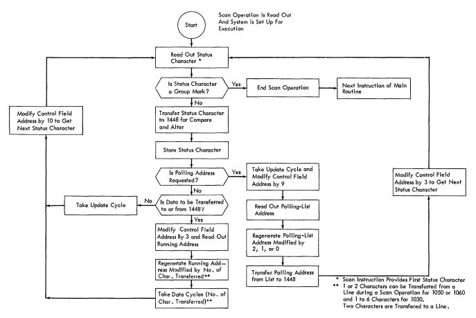
Figure 8. Flow Chart of Scan Operation
