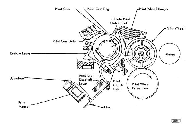
Figure 2-2. Printing Mechanism
