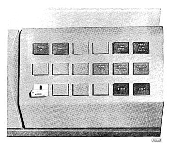
Figure 1-3. Operator Control Keys and Lights
