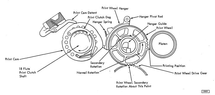
Figure 2-6. Print Wheel Operation
