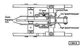
Figure 2-14. Carriage Interposer Operation
