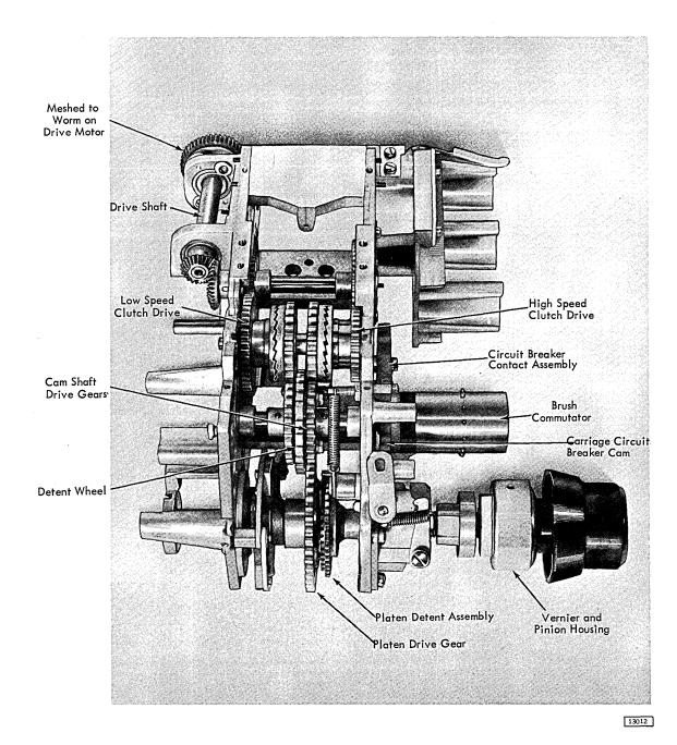
Figure 2-13. Carriage Drive Unit (Removed from Carriage)
