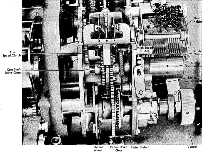
Figure 2-15. Carriage Drive Unit
