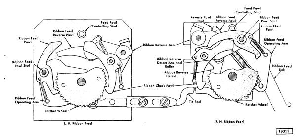
Figure 2-12. Ribbon Feed Mechanism (Feeding to Left)
