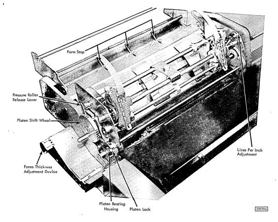
Figure 1-5. Left Side of Carriage
