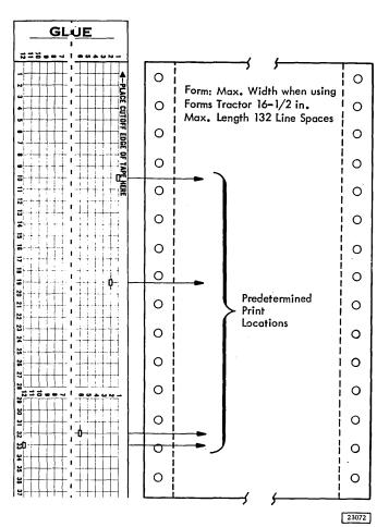
Figure 1-6. Control Tape Punching for Predetermined Printing Locations
