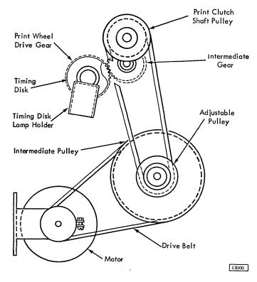
Figure 2-1. Motor and Drive (Left end view)
