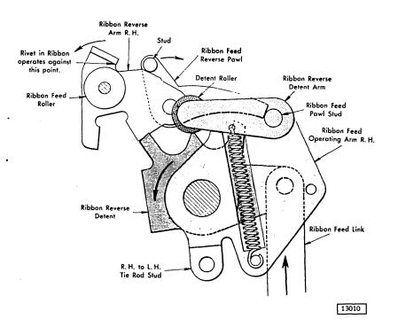
Figure 2-11. Ribbon Reversing Mechanism
