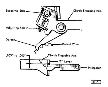
Figure 4-28. Clutch Engaging Arm
