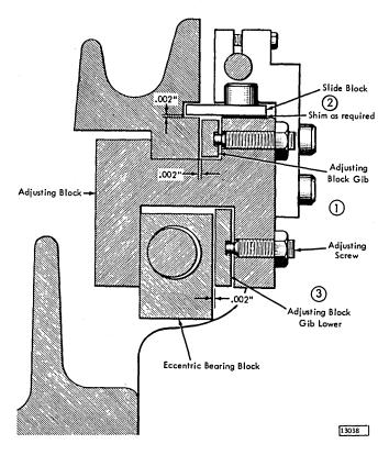
Figure 4-19. Carriage Gibs and Blocks
