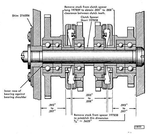
Figure 4-33. Carriage Drive Clutches
