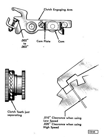
Figure 4-29. Clutch Engaging Arm Cam Plate
