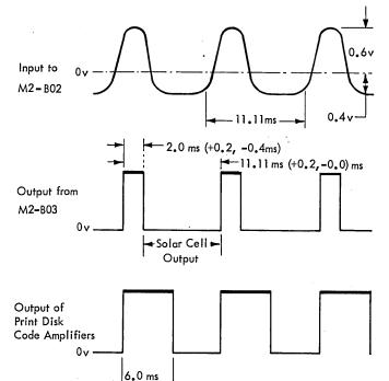
Note: Shown with print disk turning at approximately 112.5 rpm which results in a print clutch shaft speed of 300 rpm.
