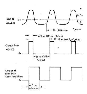
Note: Shown with print disk turning at approximately 112.5 rpm which results in a print clutch shaft speed of 300 rpm.
