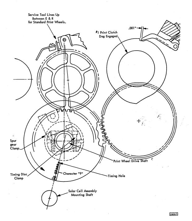
Figure 4-8. Print Wheel and Emitter Disk Timing
