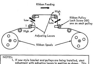
If new style bracket and pulleys are being installed, start adjustment with adjusting levers in position as shown. This provides the ribbon pulleys a vertical starting position.
