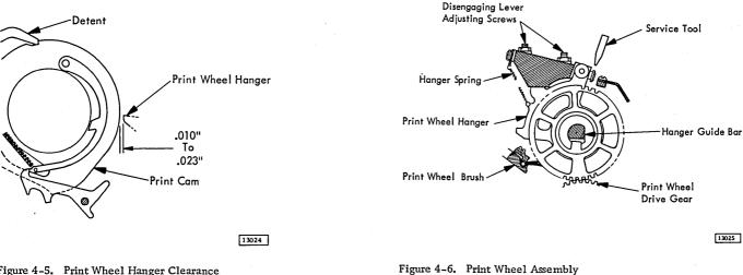
Figure 4-5. Print Wheel Hanger Clearance
