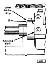
Figure 4-20. Retaining Strip
