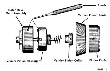
Figure 4-38. Carriage Vernier
