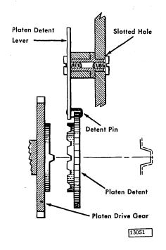
Figure 4-32. Platen Clutch Detent
