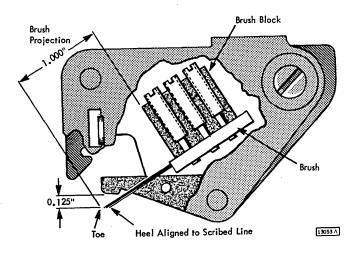
Figure 4-34. Carriage Tape Brush Alignment
