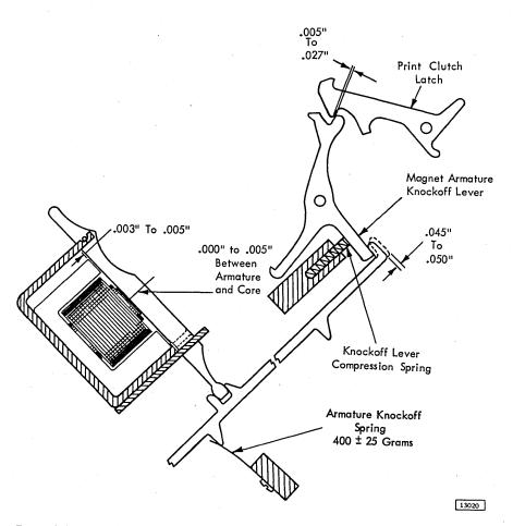
Figure 4-1. Print Magnet Armature and Link
