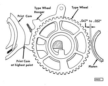
Figure 4-15. Print Wheel to Platen Clearance
