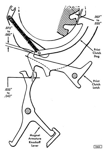
Figure 4-2. Print Clutch Latch
