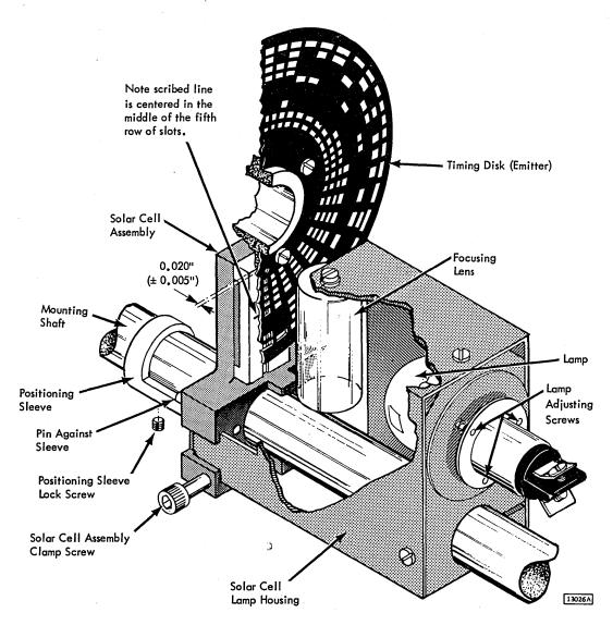
Figure 4-7. Timing Disk and Solar Cell Assembly
