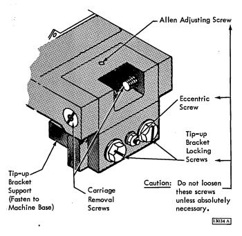
Figure 4-14. Carriage Platen Alignment
