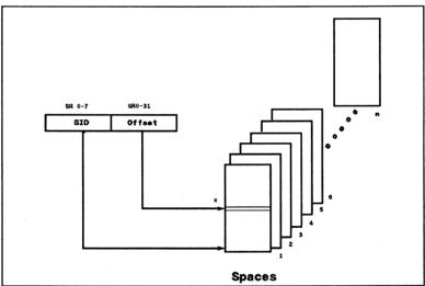
Figure 1. HPPA Spaces and Space/Offset Registers.
