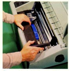
Clean, modular design allows easy ribbon cartridge replacement
