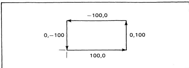
Beginning at the current pen position, a series of vectors is drawn by moving the pen 100 units to the right, up 100 units, left 100 units, and finally down 100 units. The same figure could have been drawn at any screen location by first positioning the pen to the desired starting point before sending the drawing sequence.
