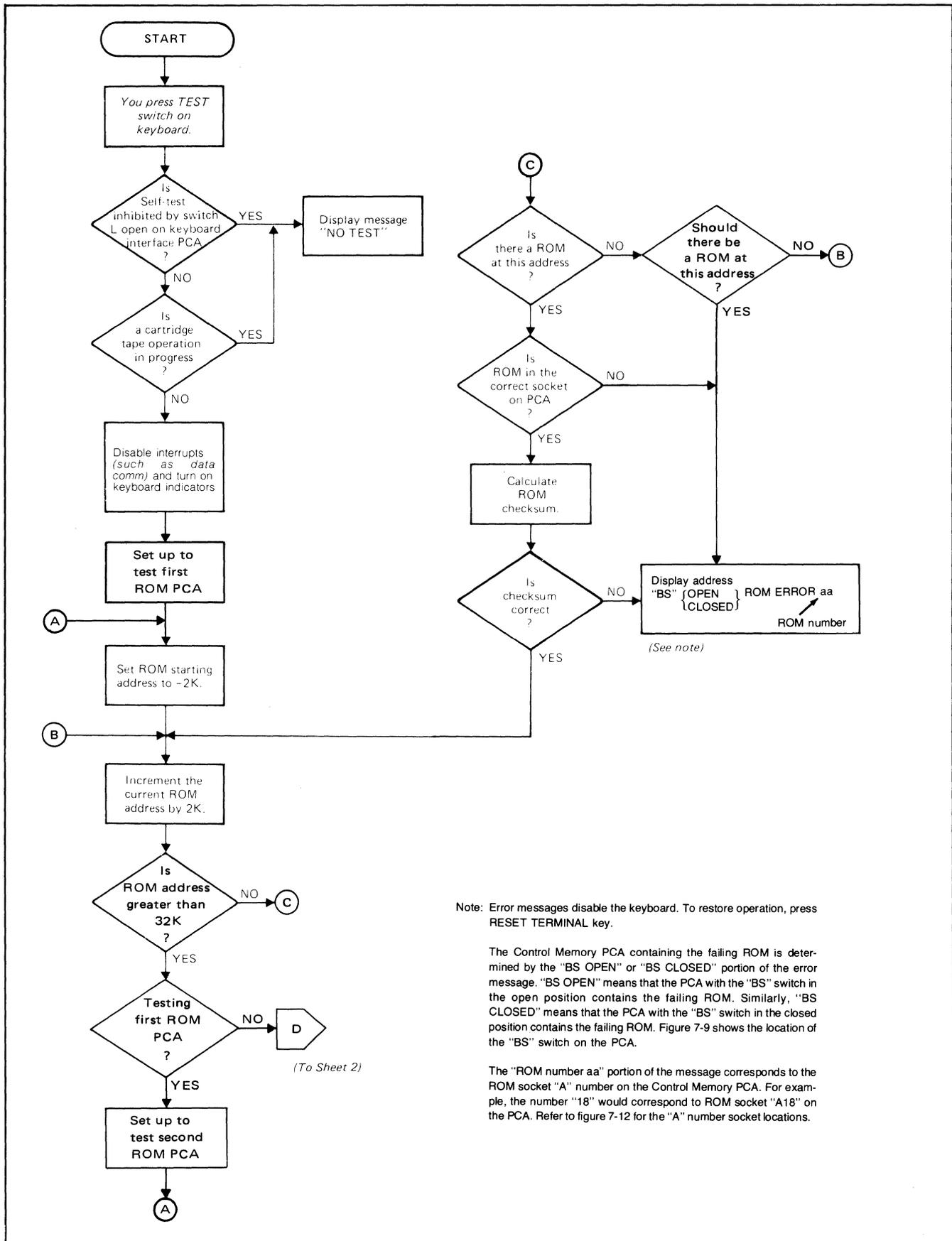
Note: Error messages disable the keyboard. To restore operation, press RESET TERMINAL key.
