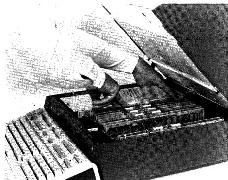
4. ( ) Reinstall the PCA into the vacated Backplane Assembly connector.
