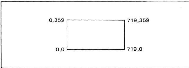
Since no format is indicated, ASCII absolute is assumed. The "a" raises the pen, which is moved to (0,0) and lowered. Vectors are then drawn to (719,0), (719,359), (0,359), and back to (0,0). (Note that the values are delimited by spaces or commas. The capital Z (a nop) terminates the sequence. Imbedded carriage return and line feed characters are ignored.
