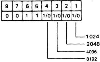
The amount of display memory (blocks of 1K) available in the terminal is returned. The amount can range from 1K to 9K bytes. The actual number of displayable characters is less than the returned figure by at least 12% minus another 500 bytes for system use.
