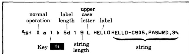
After the key assignment in the previous example has been made, a display of the key assignments would appear as follows:
