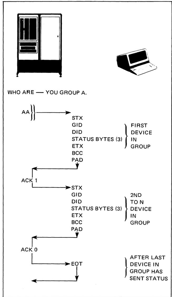
Figure 5-15. Typical Configuration Status Request and Response Sequence
