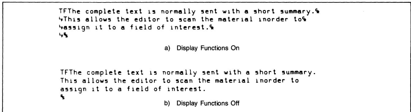
Figure 5-24. Control Character Display On Driver Terminal
