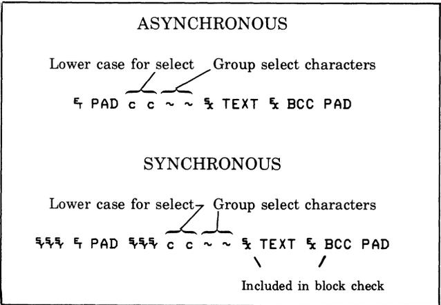
**Line Select.** A "line select" allows you to select all of the terminals on a communication line. This is also known as "Broadcast" mode. Both the group and device id characters are replaced with tildes (~).
