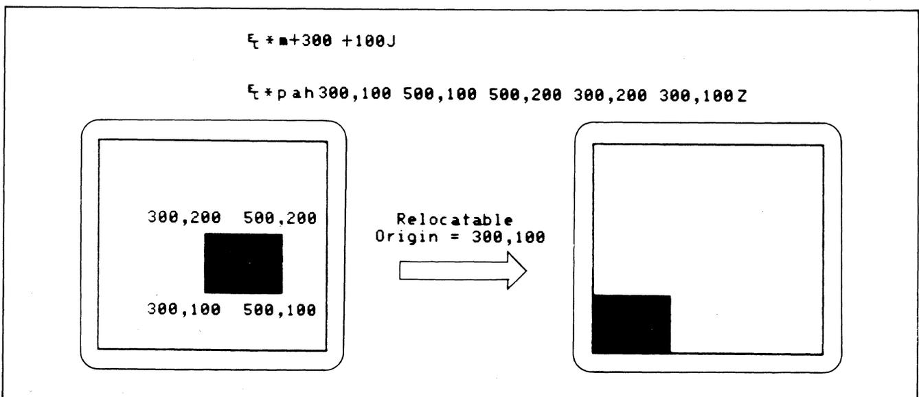
**SET RELOCATABLE ORIGIN TO CURRENT PEN POSITION.** The relocatable origin can be set to the current pen position.
