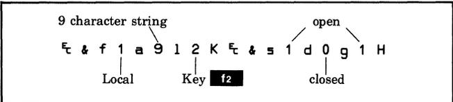
The soft keys can be used to hold log-on, program control, and log-off messages. This makes it easier for the terminal operator to use unfamiliar computer systems.
