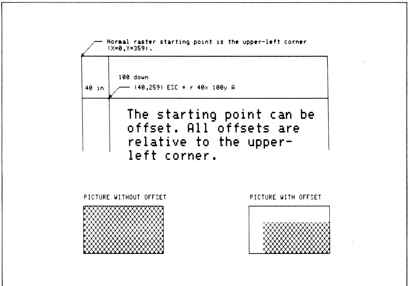
Figure 3-11. Raster Data X and Y Offsets
