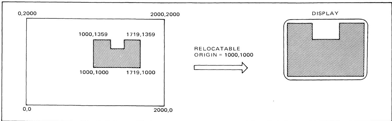
Figure 3-7. Relocatable Origin
