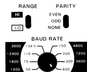
Figure 5-13. Block Keyboard Data Communication Switches
