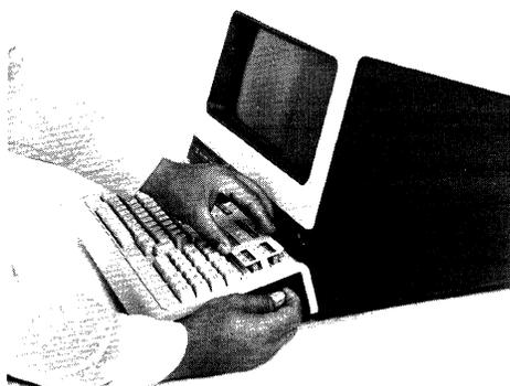
A. REMOVING A KEYBOARD OVERLAY
