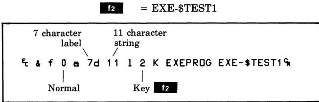
A third key could be used to log off of the system:
