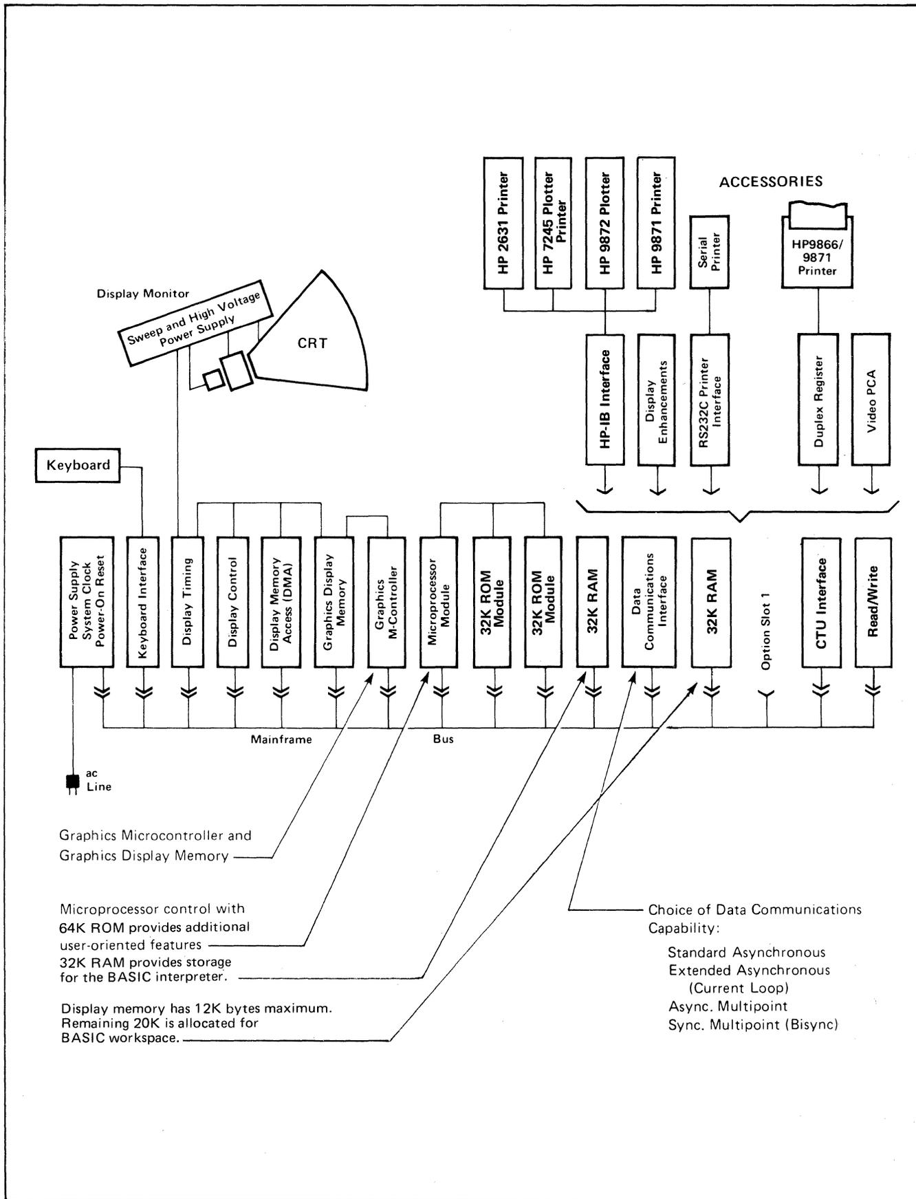
Figure 1-1. Terminal Architecture
