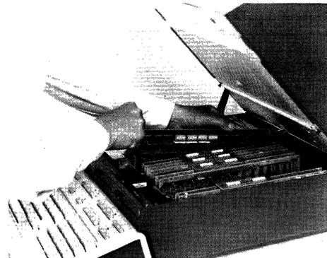
2. ( ) Locate the particular PCA, and remove the cable hood connector from the PCA. Then, remove the PCA from the Backplane Assembly connector.
