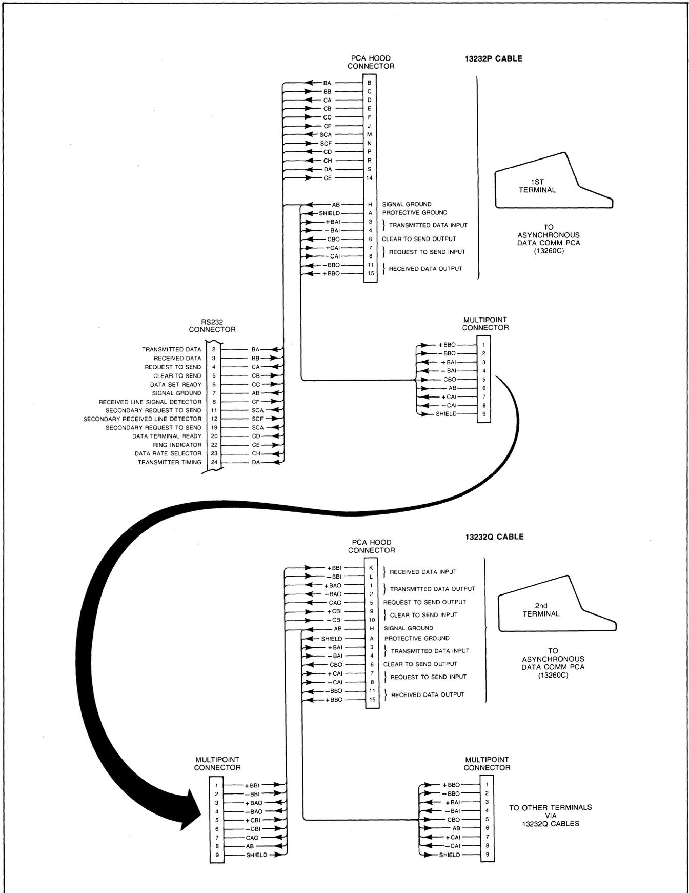
Figure 7-22. Asynchronous Multipoint Cabling
