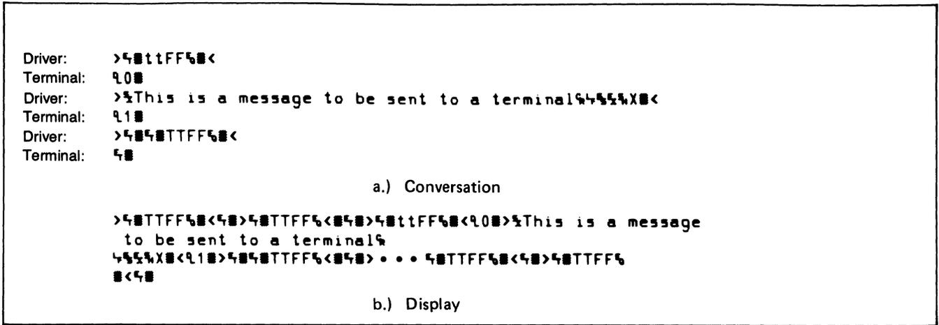
Figure 5-23. Sample Select Sequence Using Driver Mode
