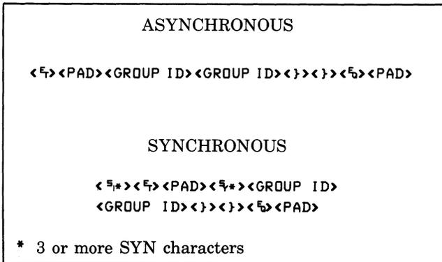
Three bytes of status information are returned for each responding terminal. Figure 5-15 shows a typical status request and responses from a terminal group.
