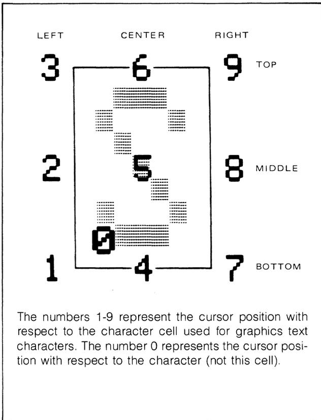
For example, if text was to be right justified and set with a base line on top of the normal character position, the number "9" would be used. Figure 3-17 illustrates the various text positions.
