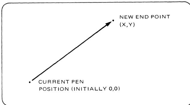
Figure 3-8. Current Pen Position And New End Point
