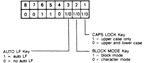
**BYTE 1 KEYBOARD INTERFACE SWITCHES (A-D)**
