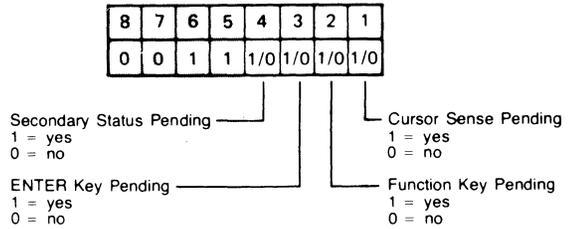
**BYTE 2 KEYBOARD INTERFACE SWITCHES (E-H)**
