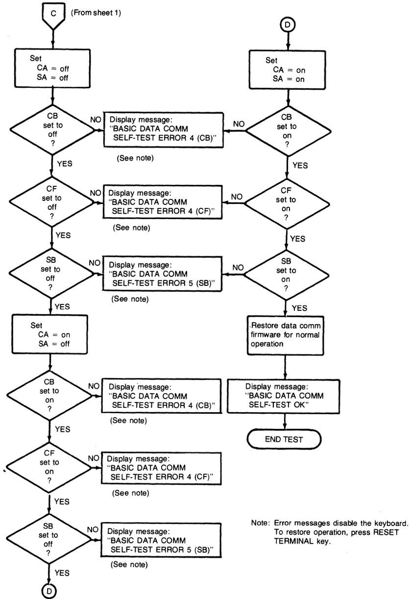
Figure 7-31. Basic Data Comm Self-Test Flowchart (Sheet 2 of 2)
