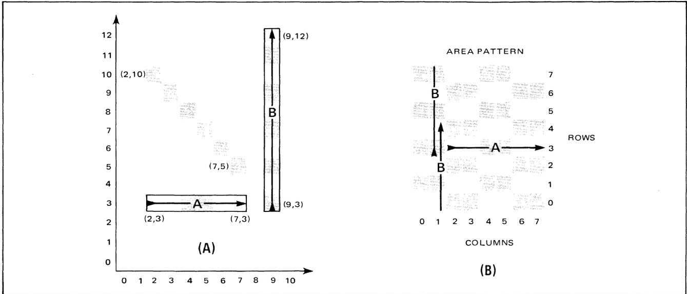
Figure 3-4. Using Area Patterns As Line Types
