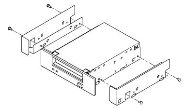
**2** Use a screwdriver to release the 5¼-inch front panel from the tape drive and remove it. Fit the 3½-inch front panel and push firmly until the panel clicks into place.
