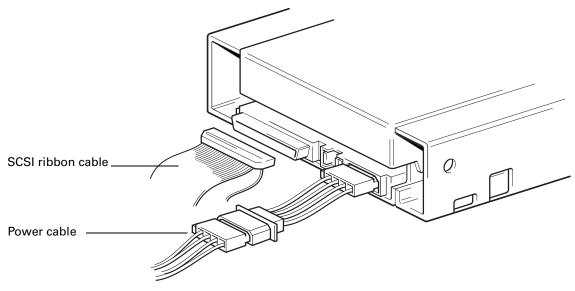
**2** Attach a spare SCSI cable to the SCSI connector.
