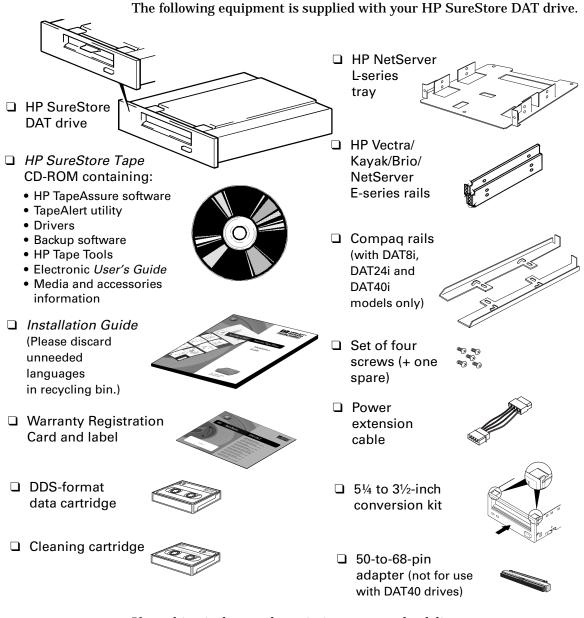
If anything is damaged or missing, contact the delivery company or your supplier. Spare jumpers for the drives' SCSI ID switch may also be supplied.
