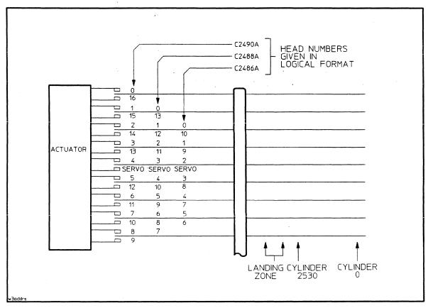
Figure 3-1. Disk Drive Addressing Structure
