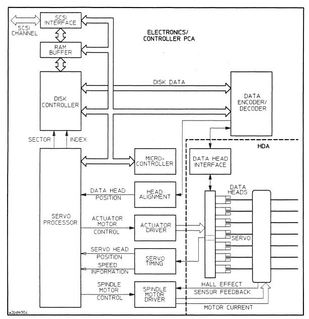
Figure 3-3. Disk Drive Block Diagram
