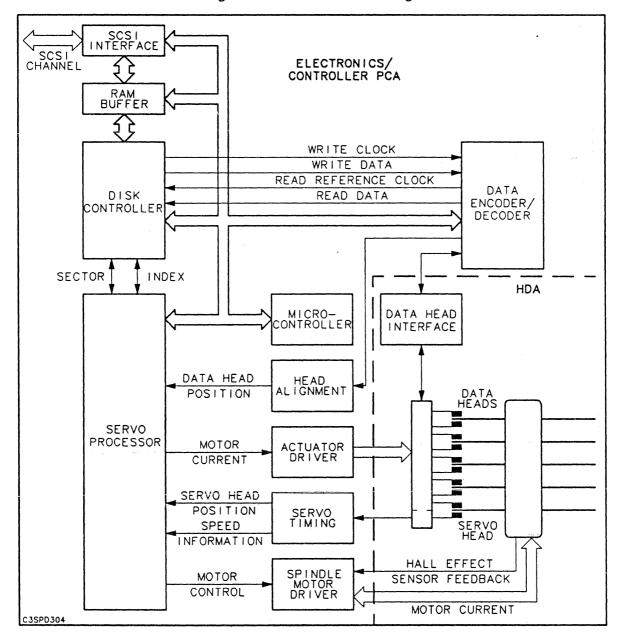
Figure 3-4. Disk Drive Block Diagram.
