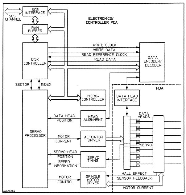
Figure 3-3. Disk Drive Block Diagram
