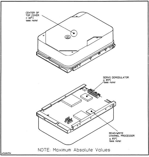
Figure 2-4. HDA Temperature Measuring Points
