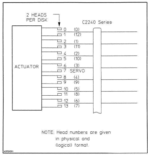
Figure 3-1. Disk Drive Addressing Structure
