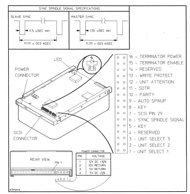
Figure E-2. Narrow, Single-Ended: Interface, Address and Option Connectors
