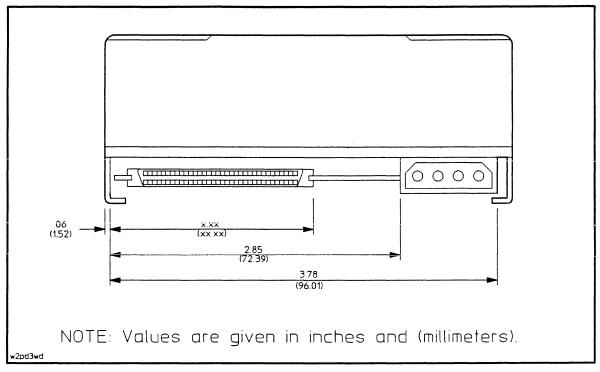
Figure G-3. Wide, Differential: Connector Dimensions
