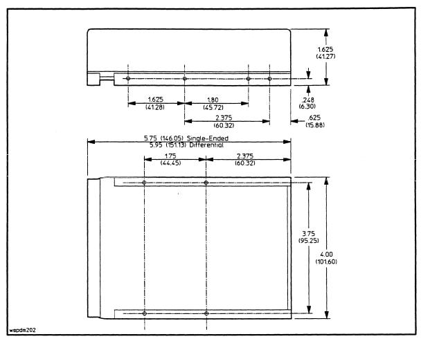
Figure 2-3. Chassis Dimensions and Mounting Locations
