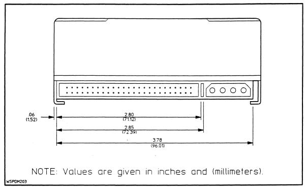
Figure E-3. Narrow, Single-Ended: Connector Dimensions
