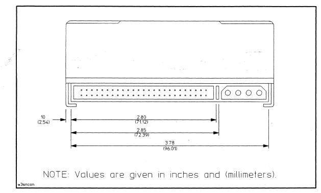
Figure E-3. Narrow, Single-Ended: Connector Dimensions
