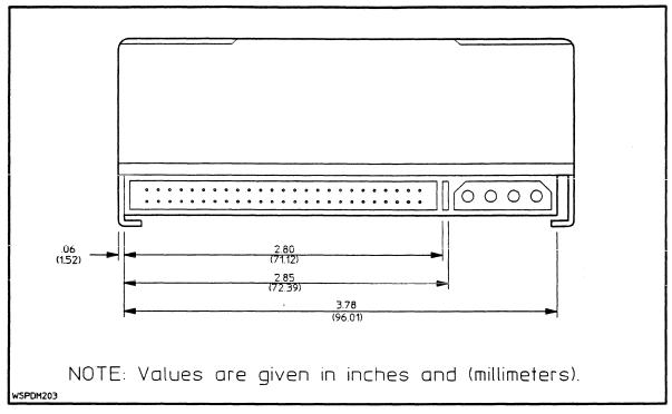
Figure F-3. Narrow, Differential: Connector Dimensions
