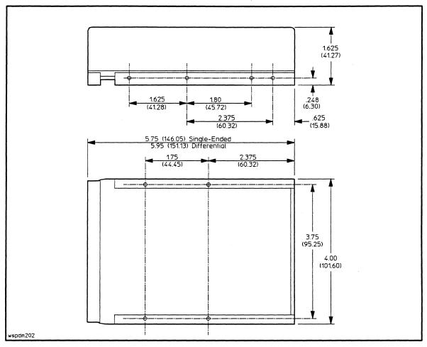
Figure G-1. Wide, Differential: Disk Drive Dimensions,
