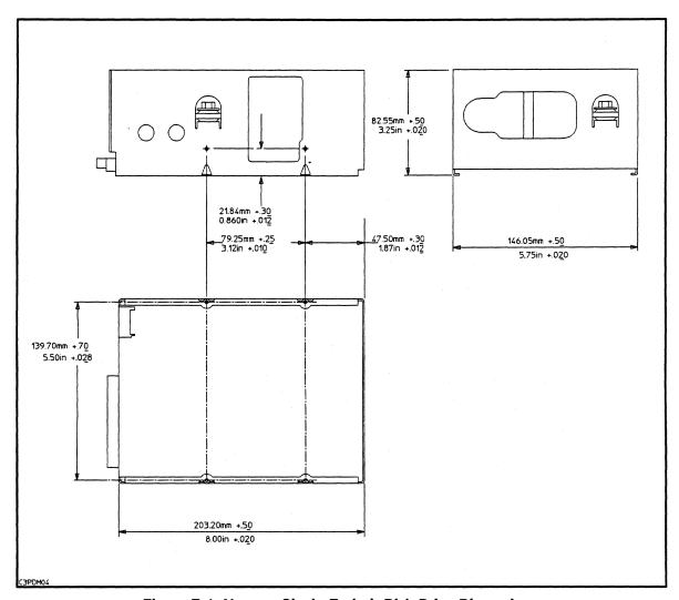
Figure F-1. Narrow, Single-Ended: Disk Drive Dimensions
