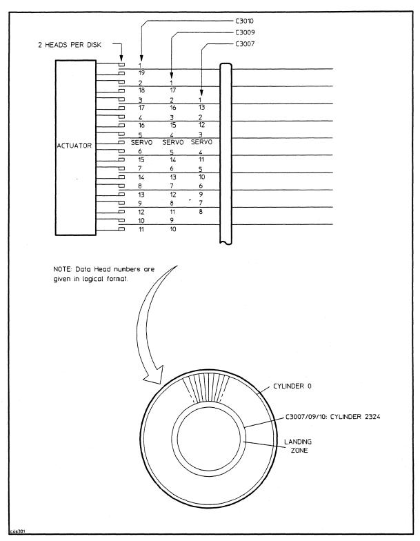
Figure 3-1. Disk Drive Addressing Structure
