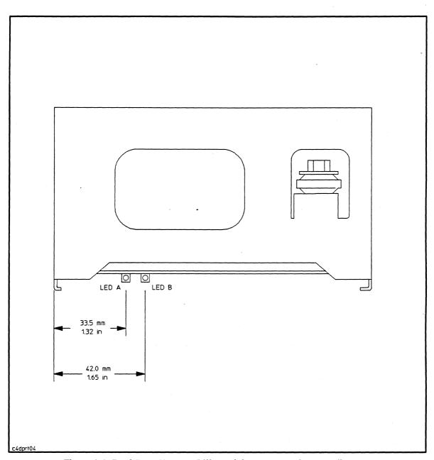
Figure I-4. Dual Port, Narrow, Differential: Front Panel LED Indicators
