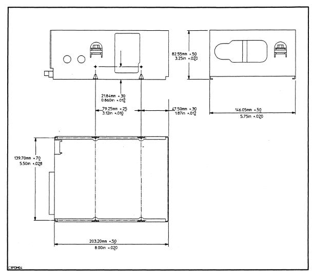
Figure 2-2. Chassis Dimensions and Mounting Locations
