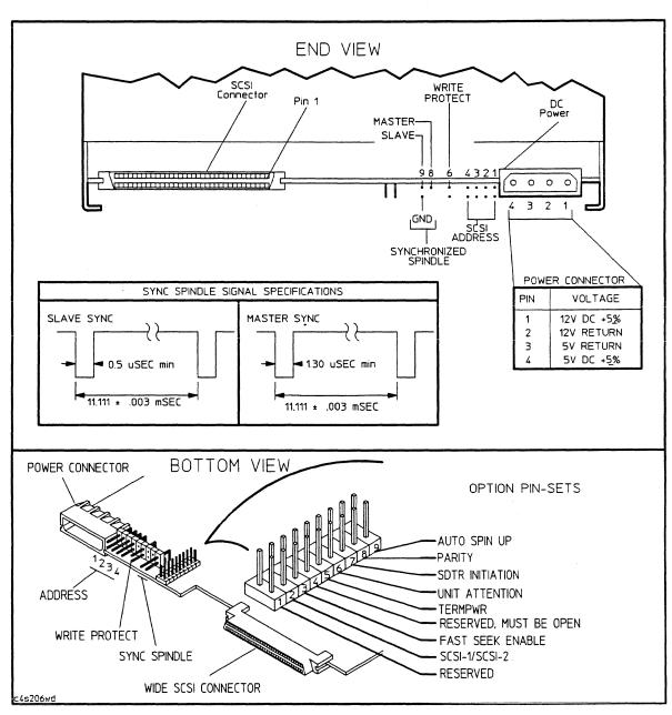
Figure H-2. Wide, Differential: Interface, Address and Option Connectors
