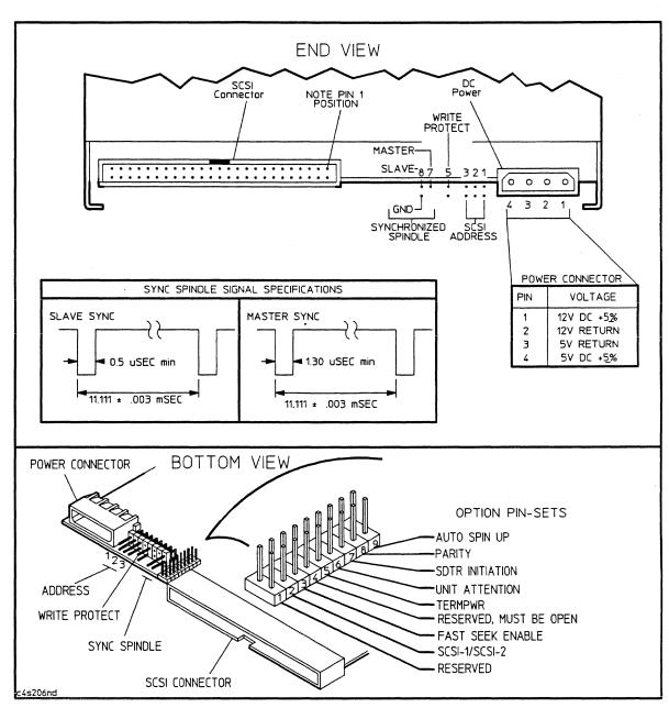
Figure G-2. Narrow, Differential: Interface, Address and Option Connectors
