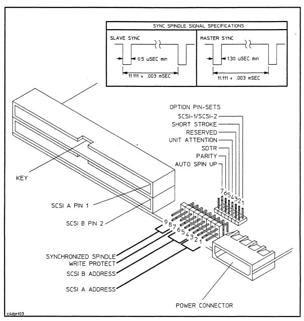
Figure I-3. Dual Port, Narrow, Differential: Interface, Address, and Option Connectors
