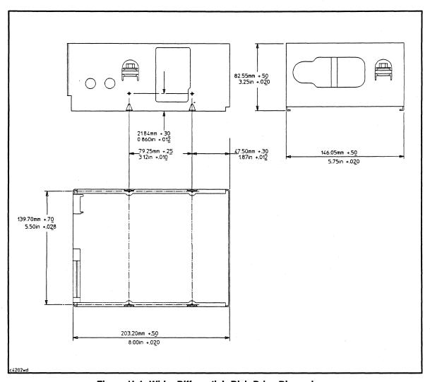
Figure H-1. Wide, Differential: Disk Drive Dimensions,
