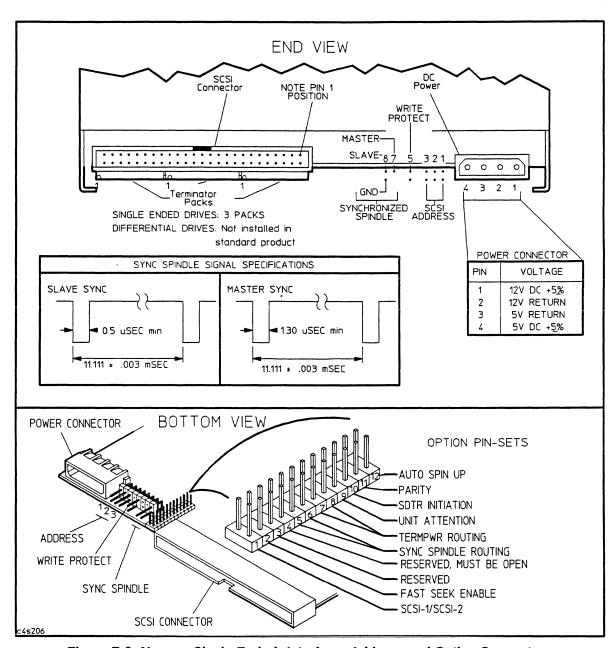
Figure F-2. Narrow, Single-Ended: Interface, Address and Option Connectors
