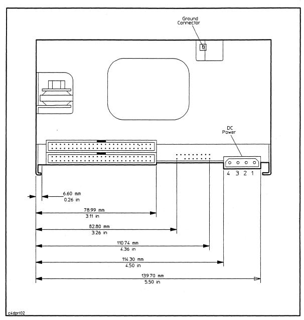
Figure I-2. Dual Port, Narrow, Differential: Connector Dimensions
