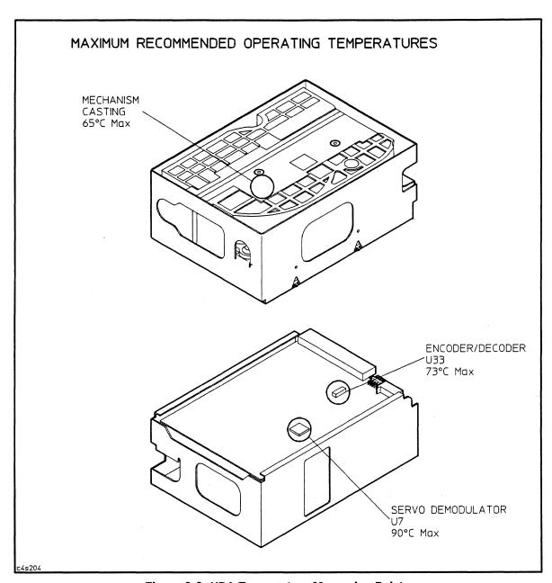
Figure 2-3. HDA Temperature Measuring Points
