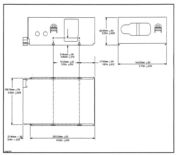
Figure I-1. Dual Port, Narrow, Differential: Disk Drive and PCA Dimensions
