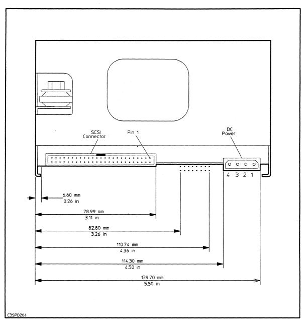
Figure F-3. Narrow, Single-Ended: Connector Dimensions
