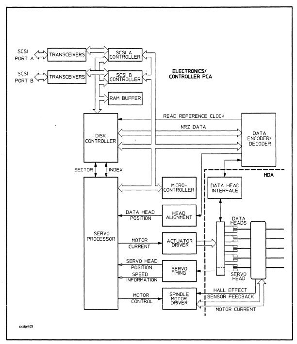
Figure I-5. Dual Port, Narrow, Differential: Drive Block Diagram
