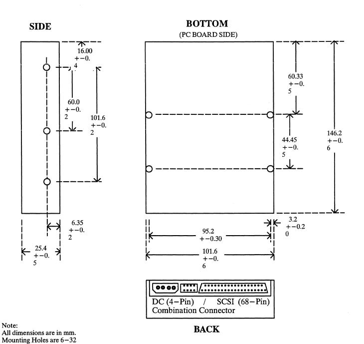
FIG. 1 DIMENSIONS AND MOUNTING
