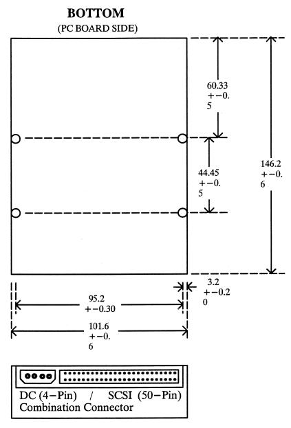
Note: All dimensions are in mm. Mounting Holes are 6-32
