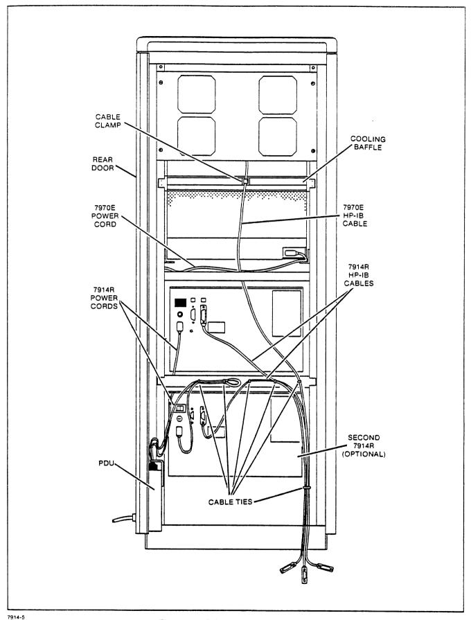
Figure 2-4. Subsystem Cable Routing
