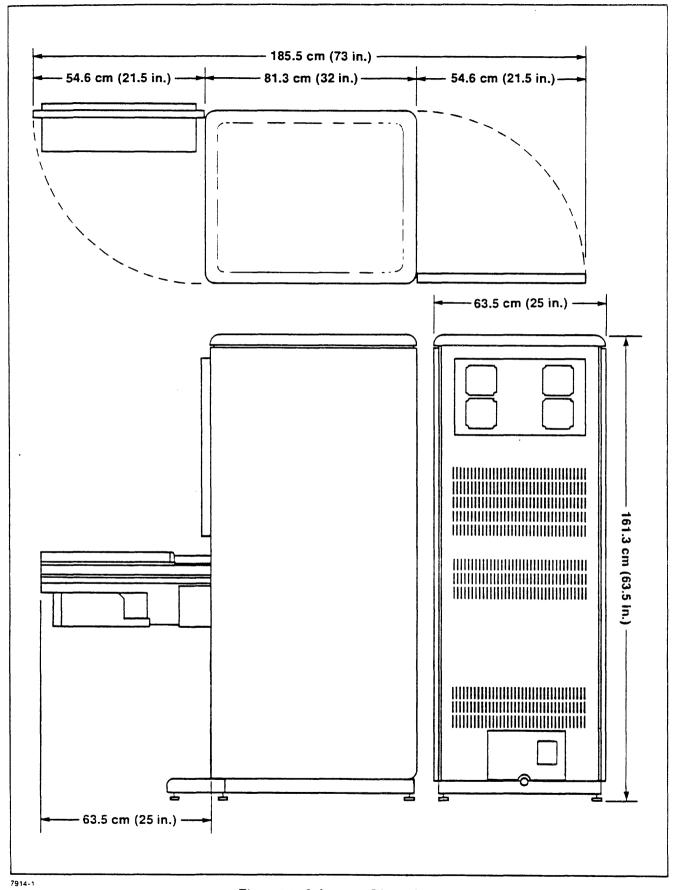
Figure 1-1. Subsystem Dimensions
