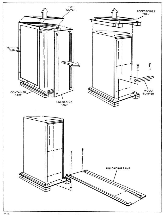
Figure 2-1. Subsystem Unpacking
