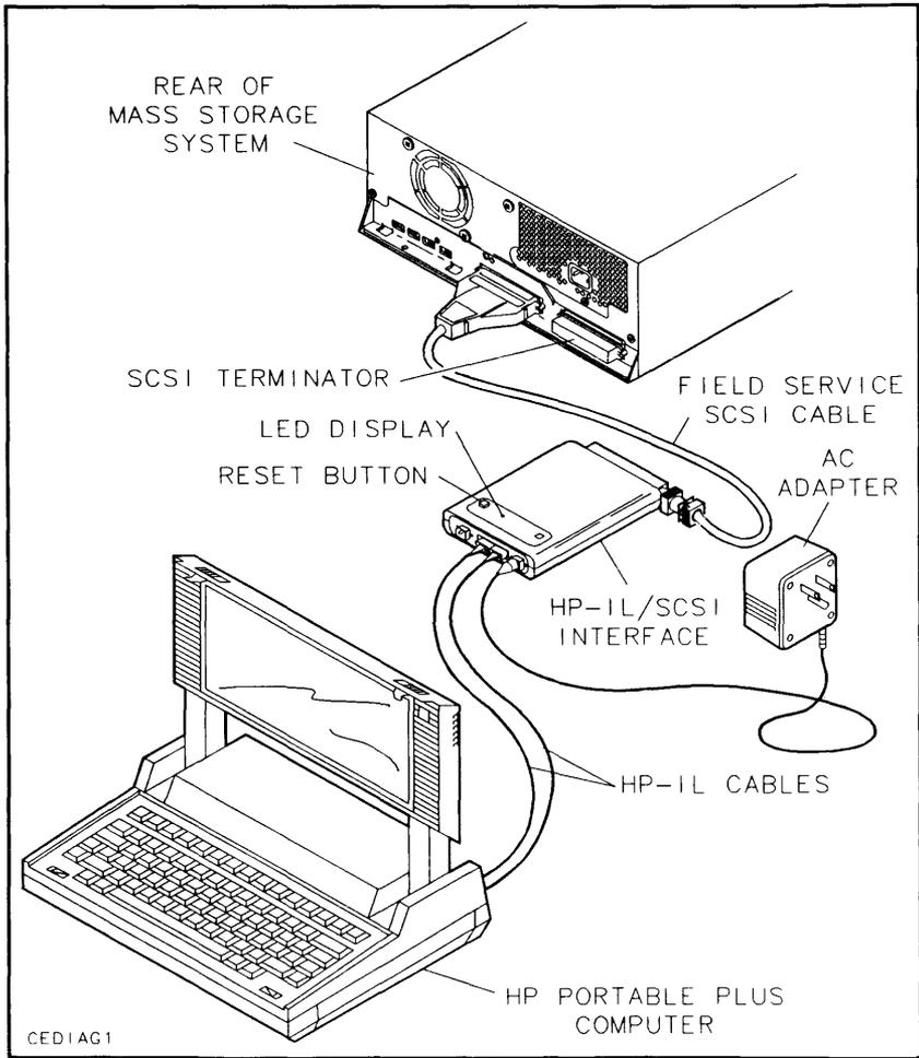
**Figure 1-1. Diagnostic Equipment Connections with Portable PLUS Only**
