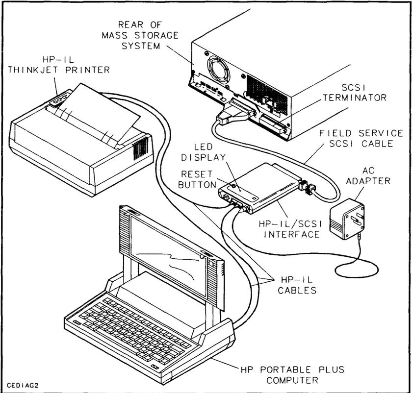
**Figure 1-2. Diagnostic Equipment Connections with Printer and Portable PLUS**
