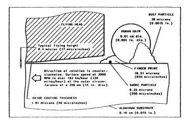
Figure 2-8. Contaminant Sizes Compared to Disk/Head Spacing
