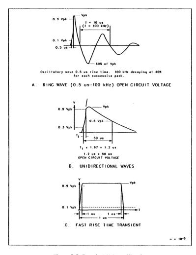
Figure 2-6. Transient Voltage Waveforms
