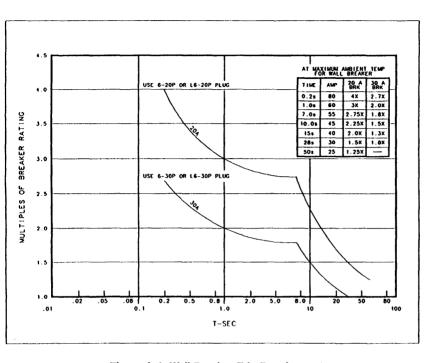
Figure A-4. Wall Breaker Trip Requirements
