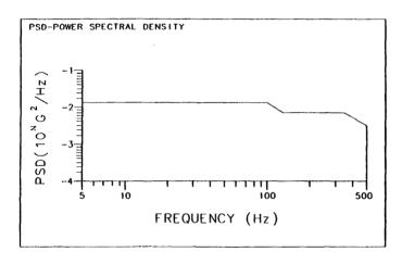
Figure 2-4. Random Vibration Profile 4: Nonoperating
