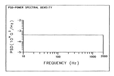
Figure 2-2. Random Vibration Profile 2: Nonoperating
