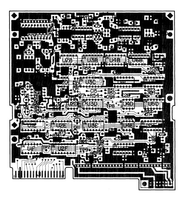
Figure 6-6. Drive Board P/N 09130-66501 Component Locator
