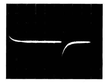
TP13 MOTOR ON Volts/DIV: .1V/DIV Time/DIV: 10ms/DIV
