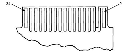
Figure 2-2: Connector J1 Pin Out (Circuit Side)
