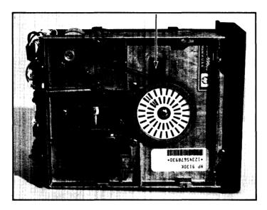
Figure 5-9: Index Detector Retaining Screw
