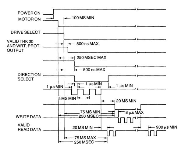
Figure 2-3: General Control and Data Timing Requirements
