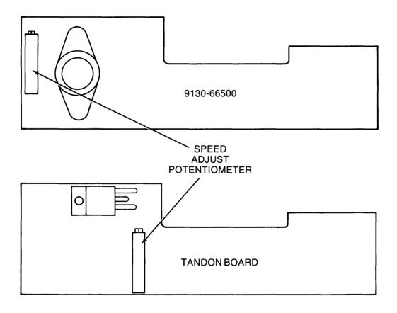
Figure 5-1: Spindle Motor Speed Adjustment
