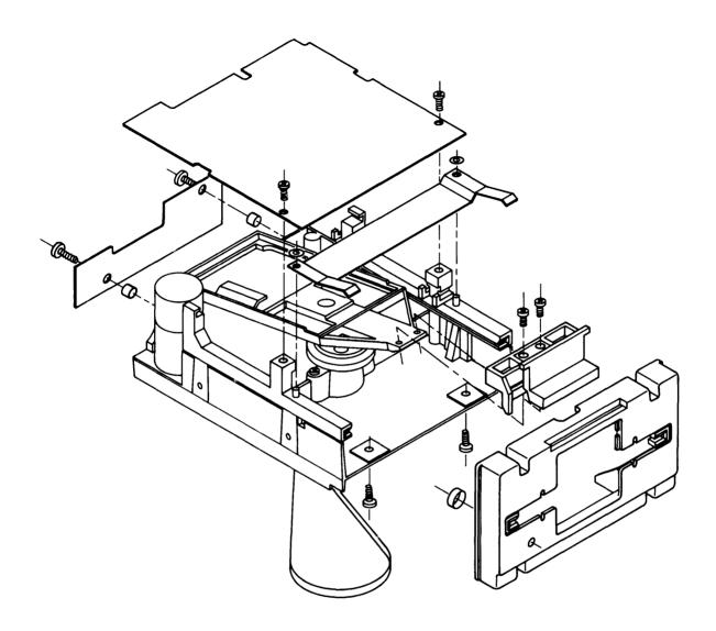
Figure 4-1: 9130K Flexible Disc Drive Exploded View
