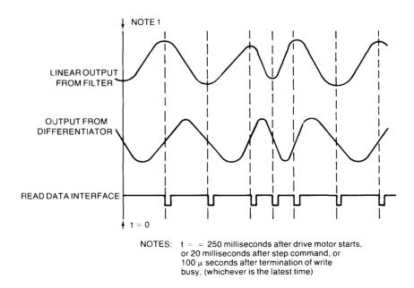
Figure 3-6: Read Timing Diagram
