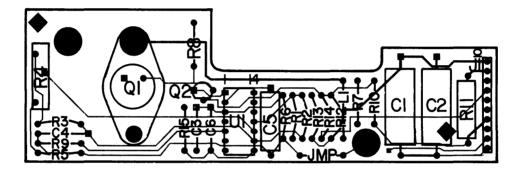
Figure 6-4. Servo Electronics Board Component Locator
