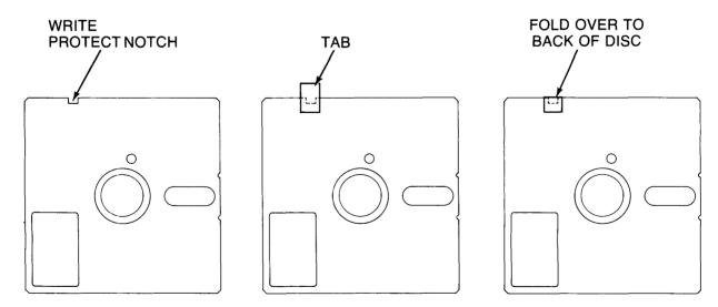
Figure 1-5. Write Protect Tab Installation
