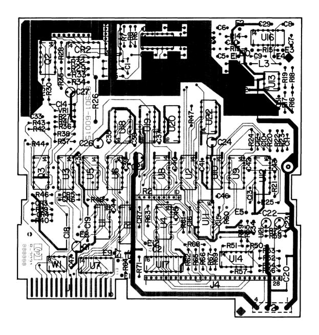
Figure 6-5. Drive Board P/N 82901-60015 Component Locator
