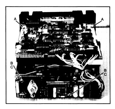
Figure 4-2: Drive Board and Servo Board Removal
