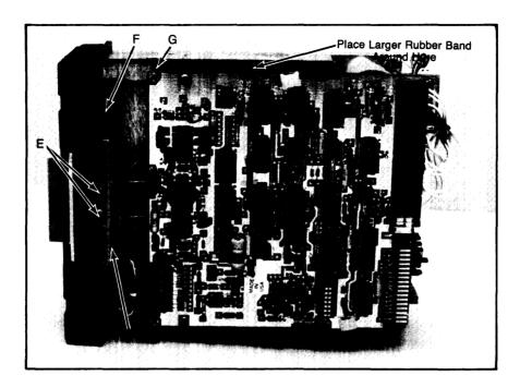
Figure 4-3: Front Panel and Latch Removal
