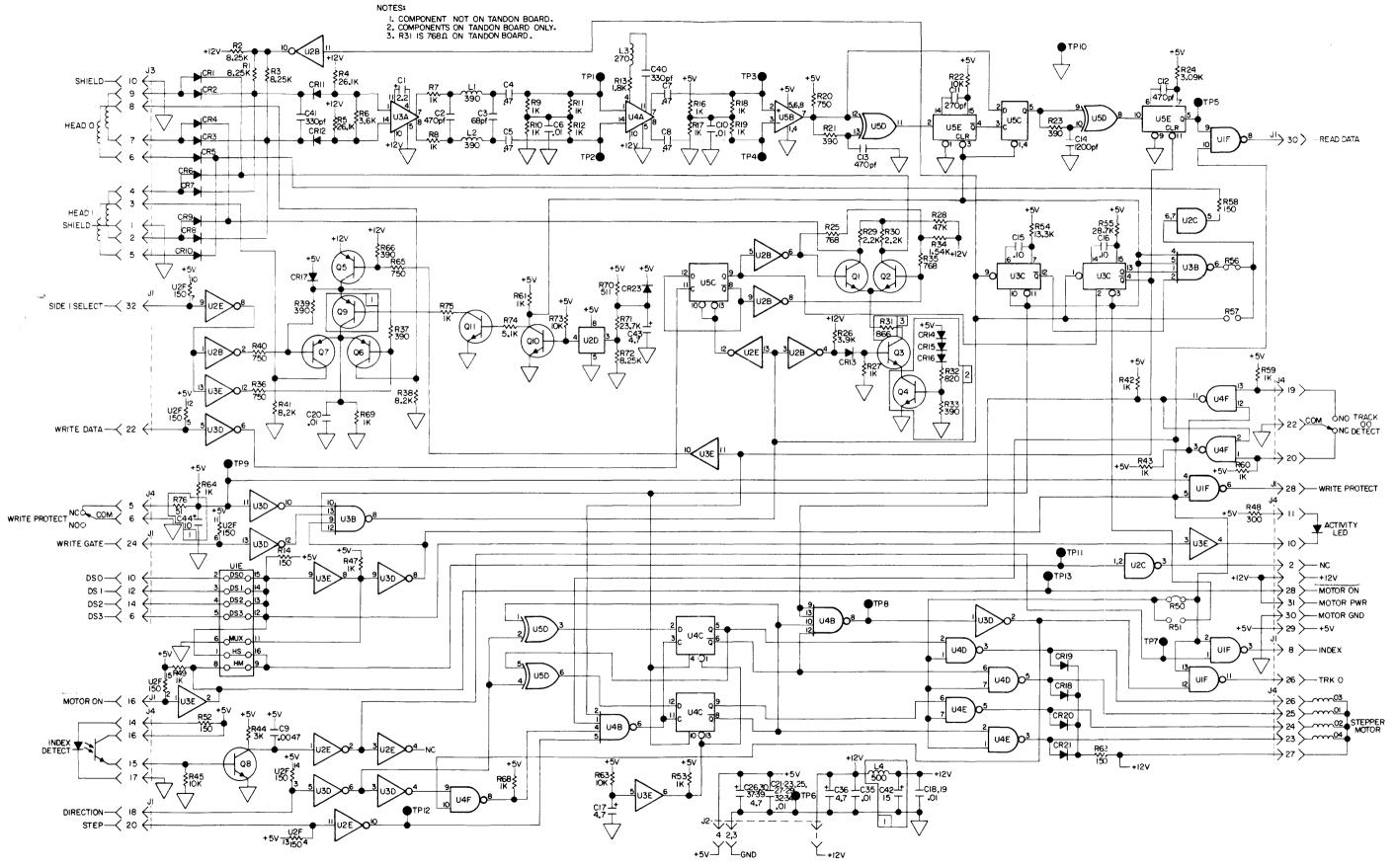
Figure 6-1: Drive Electronics Board P/N 09130-66501 Including Tandon Variations
