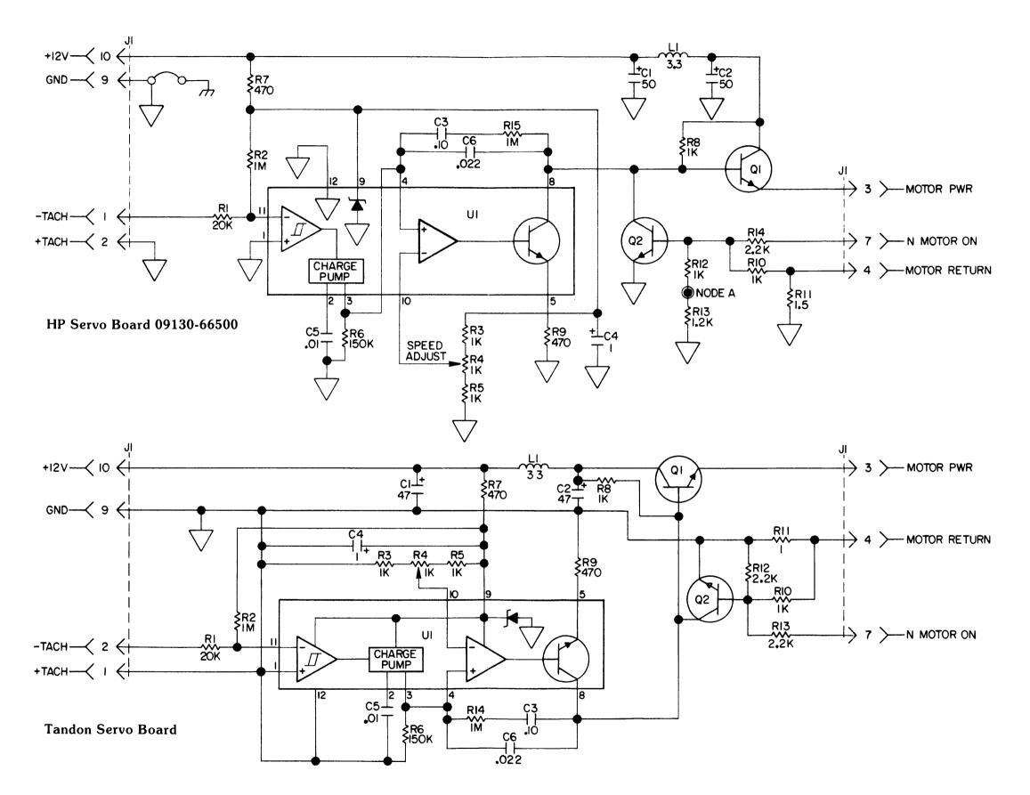
Figure 6-3: Servo Electronics Board P/N 09130-66500 Including Tandon Varitions
