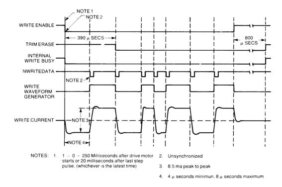
Figure 3-5: Write Timing Diagram
