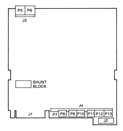
Figure 2-4: Connector Location
