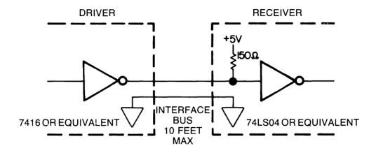
Figure 2-8: Typical Interface Driver/Receiver Circuit
