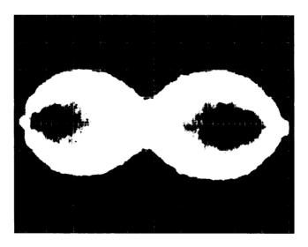
Figure 5-4: Radial Head Alignment Waveform
