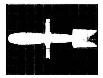
Figure 5-10. Index to Burst Waveform
