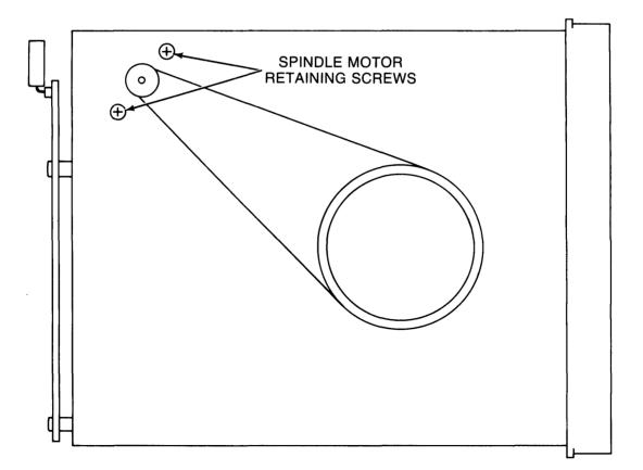
Figure 5-2: Spindle Drive Belt Adjustment
