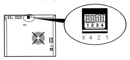
Figure 2-4. HP-IB Address Setting
