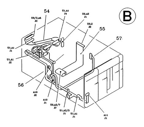
Figure 8-3. HP 35401A Cabling Layout (sheet 3 of 3)
