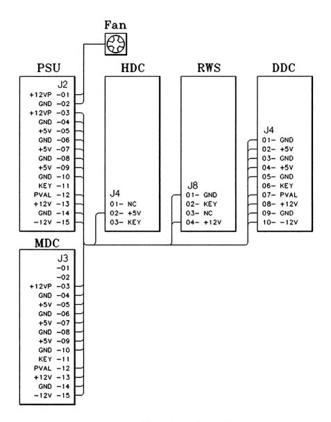
Figure 9-1. Cabling Diagram (sheet 1 of 4)
