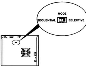
Figure 3-1. The Mode Select Switch
