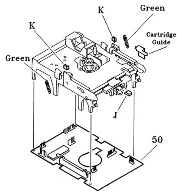
Figure 9-3. Replacement Drive Mechanism
