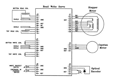
Figure 9-1. Cabling Diagram (sheet 3 of 4)
