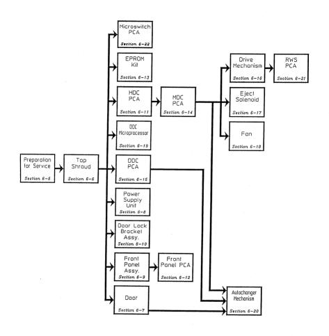
Figure 9-2. Order of Disassembly
