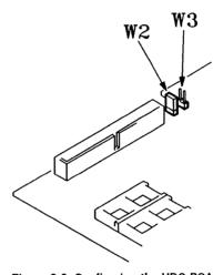
Figure 3-2. Configuring the HDC PCA
