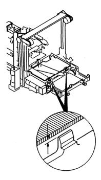
Figure 6-2. Checking the Platform Assembly
