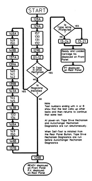
Figure 5-1. Self-Test Sequence Flowchart (See Table 5-2. for a description of individual tests.)
