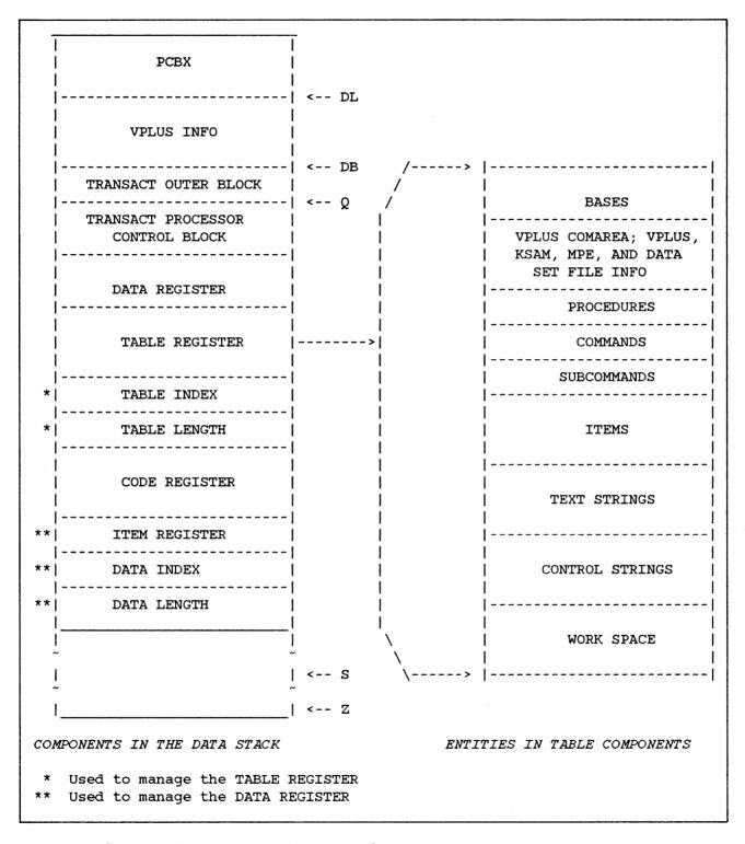
Figure E-1. Data Stack Layout for Nonsegmented Transact Program
