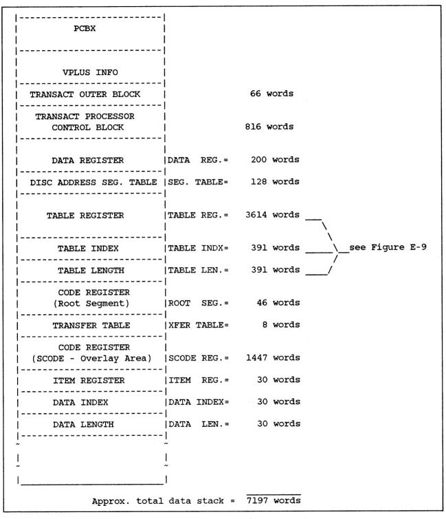
Figure E-8. Data Stack of Segmented Program
