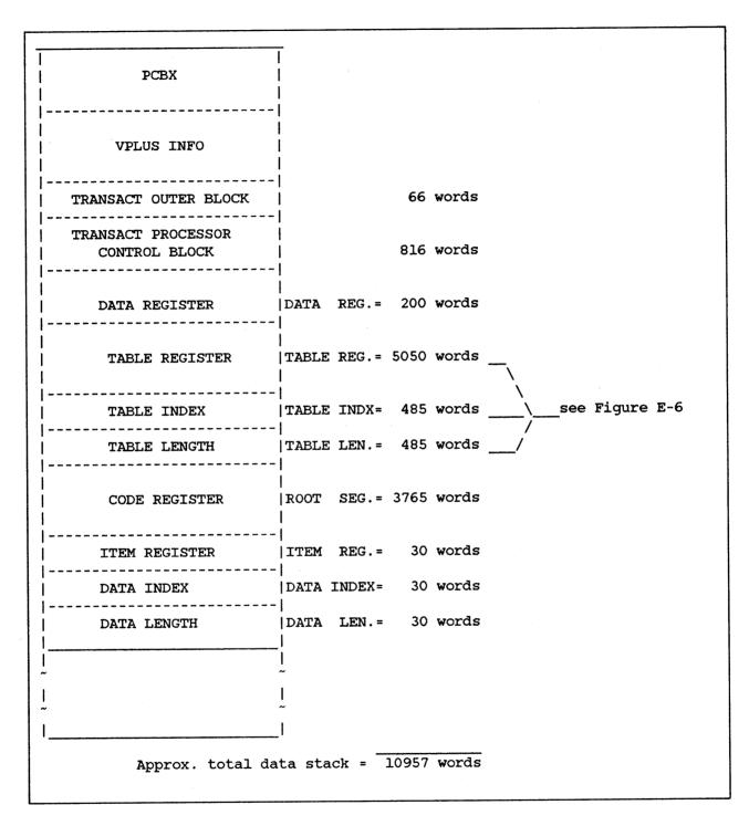
Figure E-5. Data Stack of Nonsegmented Program
