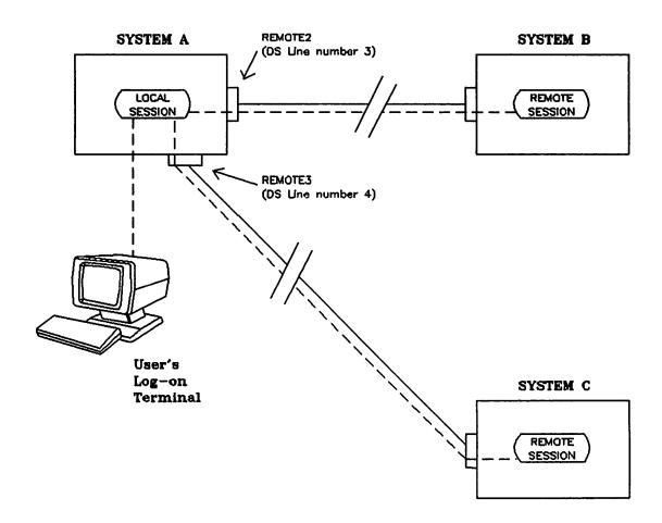
Figure 2-16. Multiple Line Example (Telephone Lines)
