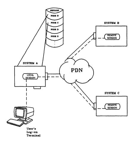
Figure 2-23. Establishing the Link With System C (X.25 Example)
