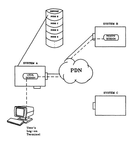
Figure 2-22. Establishing the Link With System B (X.25 Example)
