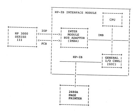
Figure 838.1 2680A Page Printer Verifier Hardware Configuration for HP 3000 Series III/HP30341A HPIB Interface
